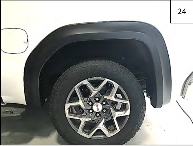
Complete Rear Flare Installation.
