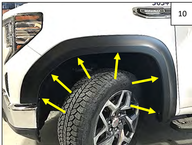
10 Press flare to fender and tighten all screws.
