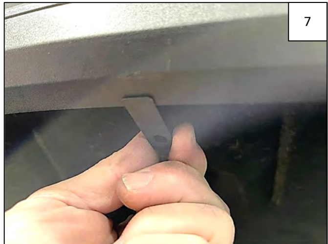
7 Remove flare from fender and slide a supplied "U" Clip over plastic lip in 4 locations, centering over marks made in Step 6.
