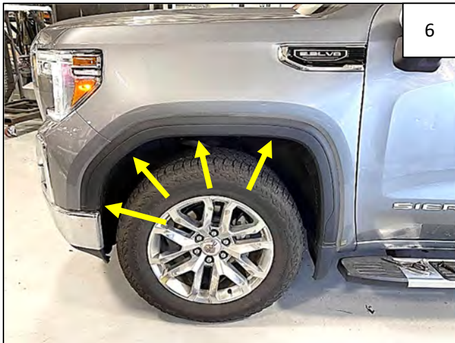
6 Hold flare firmly on vehicle. Using a grease pencil, mark 4 hole locations through flare onto fender lip.
