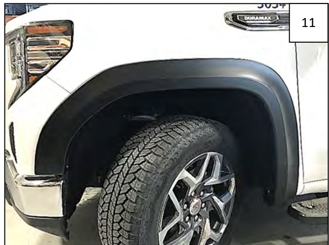
11 Complete Front Flare Installation.
