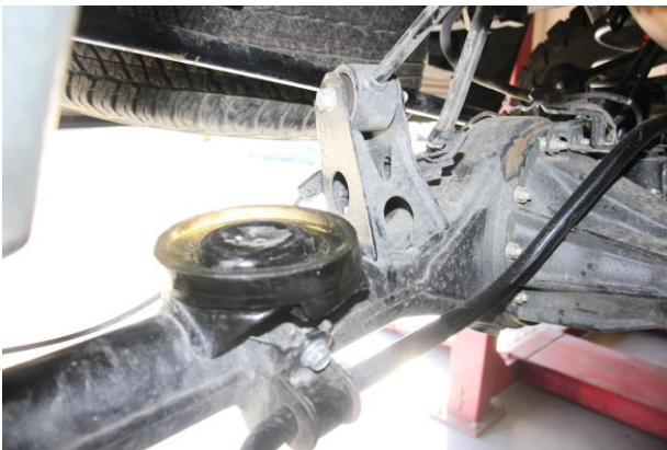
11. Install the provided urethane adapter to the spring mount on the axle, lining up the helical rise on the adapter with helical rise on the axle as shown.
