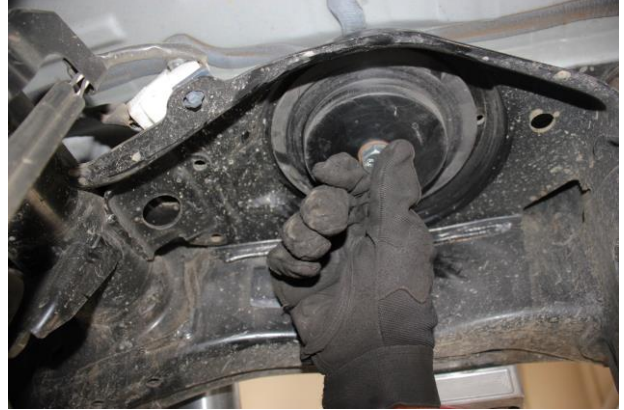
10. Install the provided spring perch adapter and secure it with the M12 x 1.75 x 30mm hex screw, and M12 washer/nut.
