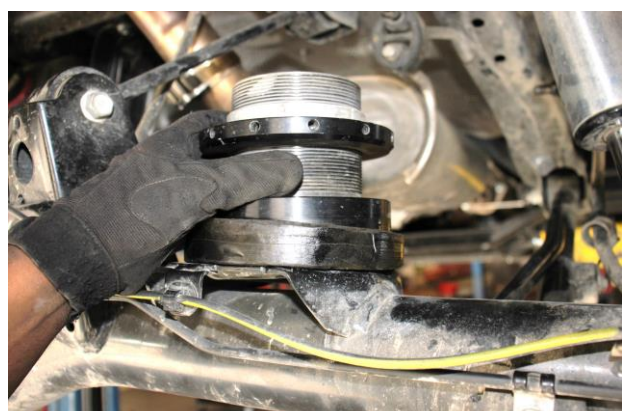
12. Install the adjustable spring perch assembly onto the urethane spring perch adapter on the axle as shown.
