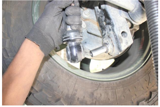
8. Remove the lower shock mount from the axle
