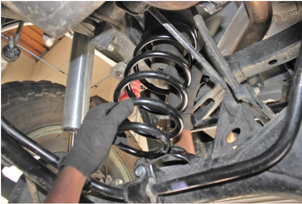
9. You can now lower the axle downward and remove the OE spring as shown. Note: Do not stretch brake lines/ABS lines, vent lines as this could cause failure of these components.
