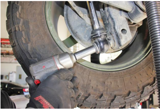
7. Loosen and remove lower shock bolt.
