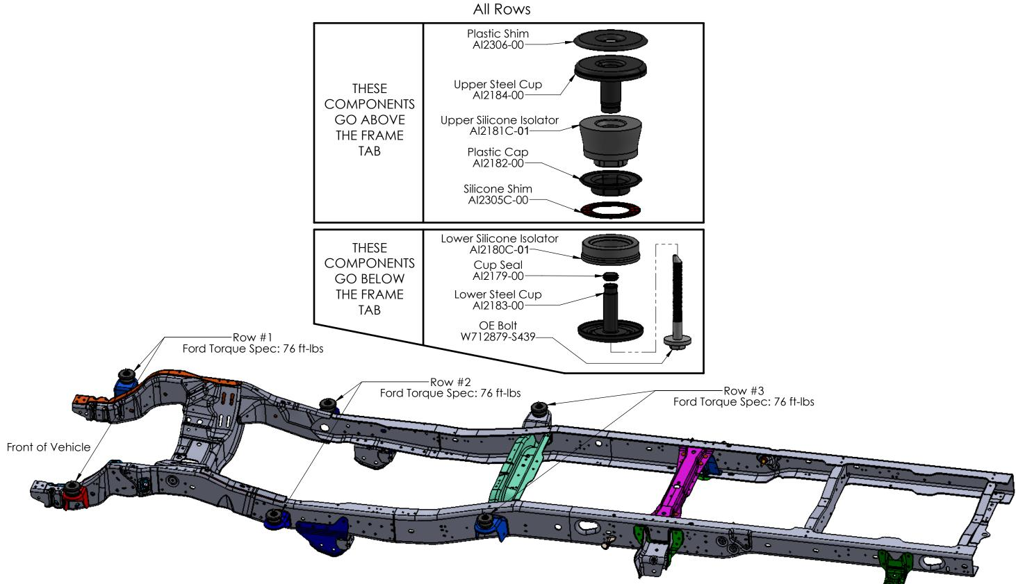
WARNING: Qualified professional installation of this product in accordance with the Ford service documentation and using a vehicle lift is required.
