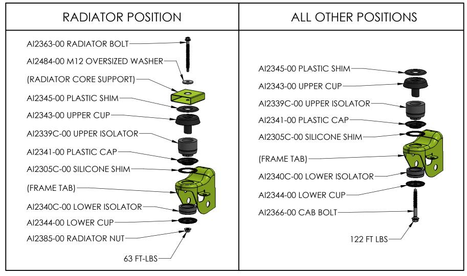
INSTALL COMPONENTS IN THE CORRECT LOCATION ACCORDING TO THIS DIAGRAM. COMPONENTS INSTALLED INCORRECTLY WILL CAUSE CLUNKING NOISE AND MAY RESULT IN DAMAGE TO THE VEHICLE. USE HAND TOOLS ONLY TO REMOVE OR INSTALL BOLTS! USING AN IMPACT WRENCH MAY RESULT IN DAMAGE TO THE BOLTS OR NUT ASSEMBLIES.
