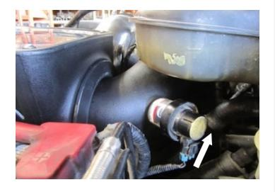
Reconnect the electrical connector to either the MAF Sensor or Temp. Sensor located on top of Tube (C).
