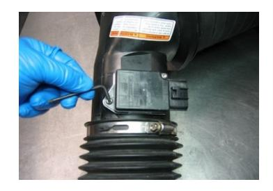
If your vehicle uses a MAF sensor, use the supplied MAF Gasket (K) and #8-32 Screws (L) to attach the MAF sensor to the Intake Tube (C). **Do not overtighten.**
