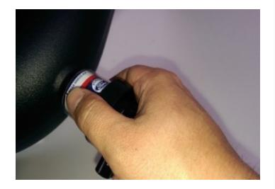
Place the Intake Tube (C) in the vehicle as shown, then rotate the Tube so the MAF sensor or Temp. sensor is facing up.
