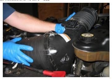
Remove the OE restriction gauge from the OE intake. Place it aside to be used later on during the install.
