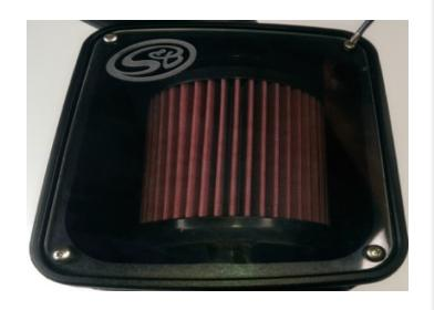
For increased air flow, we recommend using the provided Inlet Cap (U). However, if you wish to cover the Air Box from possible engine bay heat, use the Clear Lid (G).
