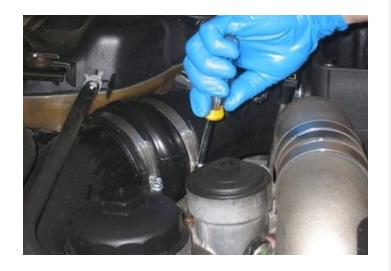
Carefully place the Air Filter (D) into the Air Box (A). Fully insert the Filter (D) on to the Intake Tube (C) and make sure the Filter is rotated and aligned so that it is evenly spaced within the Air Box. Tighten the #80 Hose Clamp (E) to secure the Filter in place.
