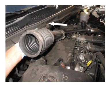
Remove the lid by first removing the latches on the side of the factory airbox.
