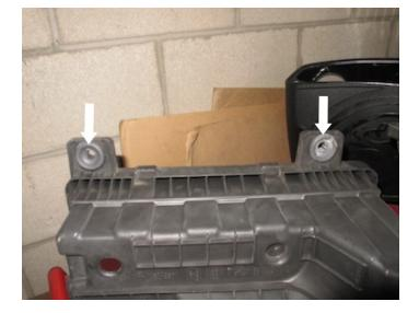
Push both grommets into part (K) Mounting Brackets. Put brackets to the side which will be used later in the install.
