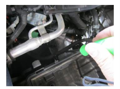
Remove the stock airbox by pulling up and out.
