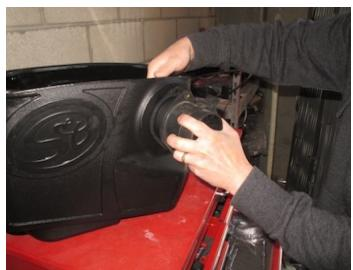
Make sure the MAF is aligned properly and that the flanges meet together.
