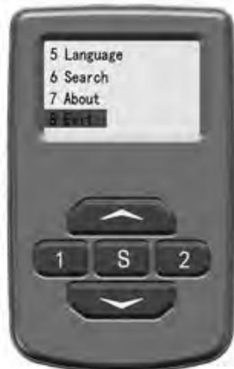
Press **↓** key to move the cursor down. and move to the "8 Exit " option, Press **S** the key to exit the setting interface.
