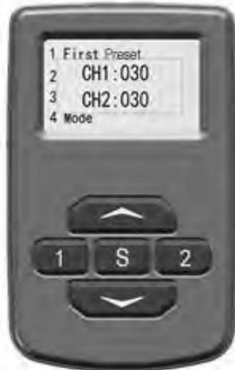
On the First Preset interface, Press **↑** and **↓** key to change the Preset PSI, and Press **1** and **2** key to change the CH1/CH2.
