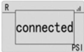
Press any button to wake up the wireless-controller. The display should show Connected. If not then please connect the controller using the Instructions below.
