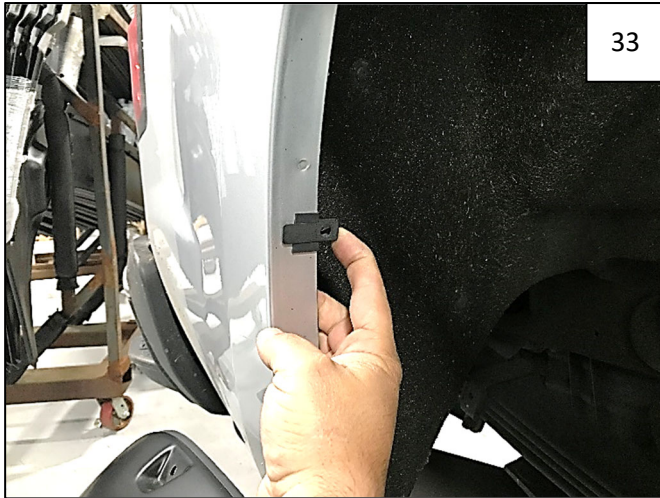
Install 5 supplied Long "U" Clips over Foam Tabs as shown.
