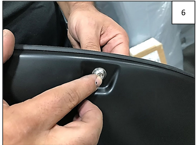
6 Insert each Bolt/Washer combination through pocket holes in flare, Bolt head and Washer on the outside.
