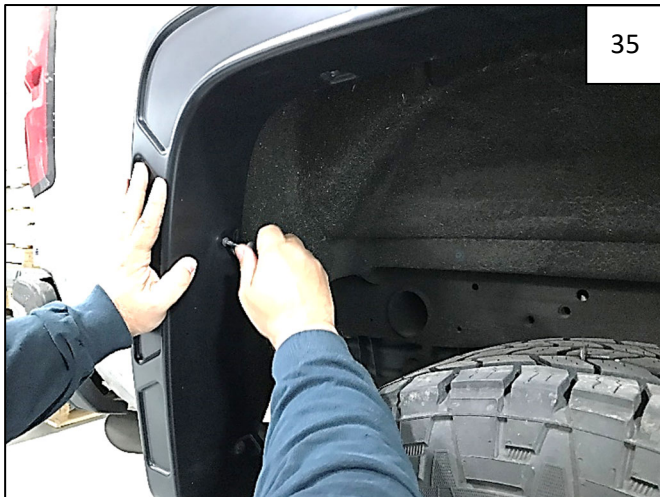
Install supplied #10 Truss Head Screws through holes in flare and into clips installed in Step 33.
