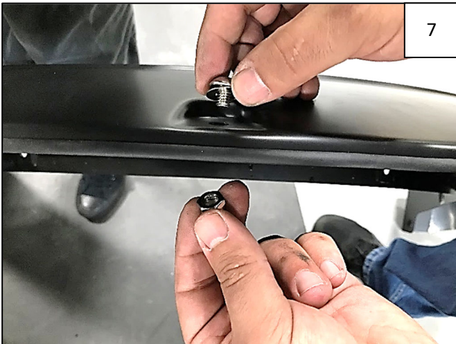
7 Place a supplied Pocket Nylock Nut over the end of each bolt and tighten using a 1/2" wrench for the Nut and the supplied T-45 Torx Bit for the Bolt. Repeat for all pockets.
