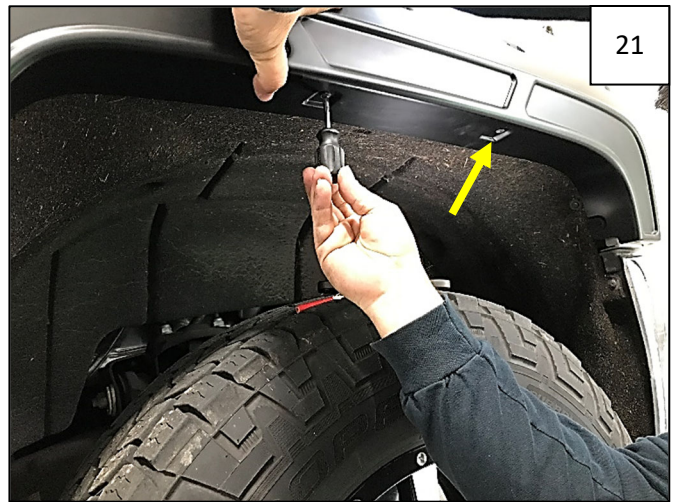
Holding flare firmly on fender, install 2 supplied #10 Truss Head Screws through topmost holes in flare and into Inner Bracket Clips. NOTE: Inner lip of flare should go over Inner Bracket installed in Steps 15-17. Do not tighten.
