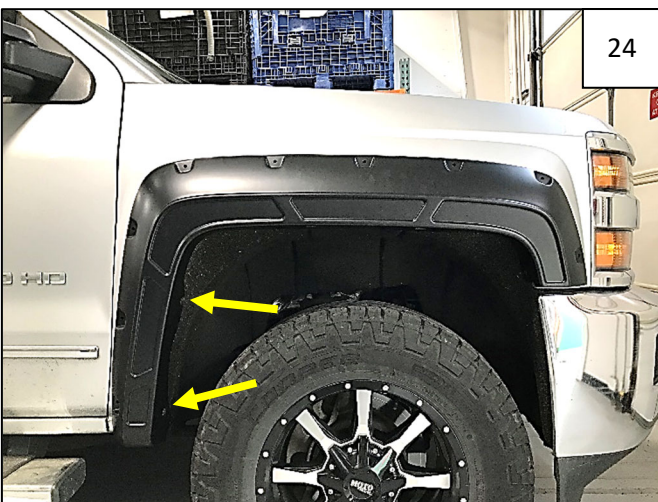
Reinstall 2 factory screws into holes at rear of flare, shown by arrows.
