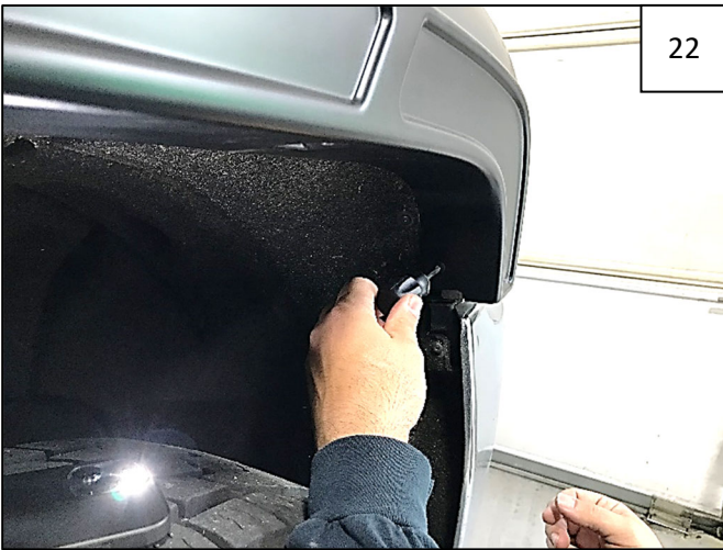
Install supplied Short Screw into "S" Clip installed in Step 20.
