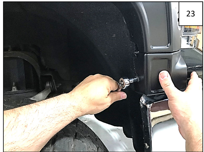
If your truck is a 2014-2015 1500, reinstall 7mm bolt removed in Step 13 through flare and into factory hole.
