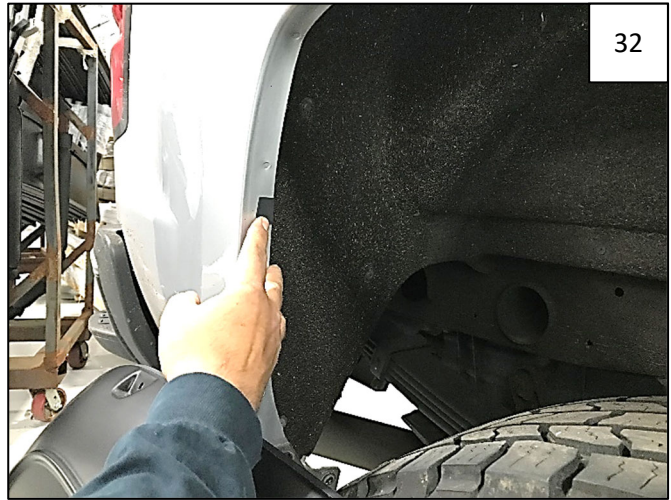
Remove flare from fender and peel liner from supplied Foam Tab. Center 5 foam tabs over marks made in Step 30, folding over wheel well lip.
