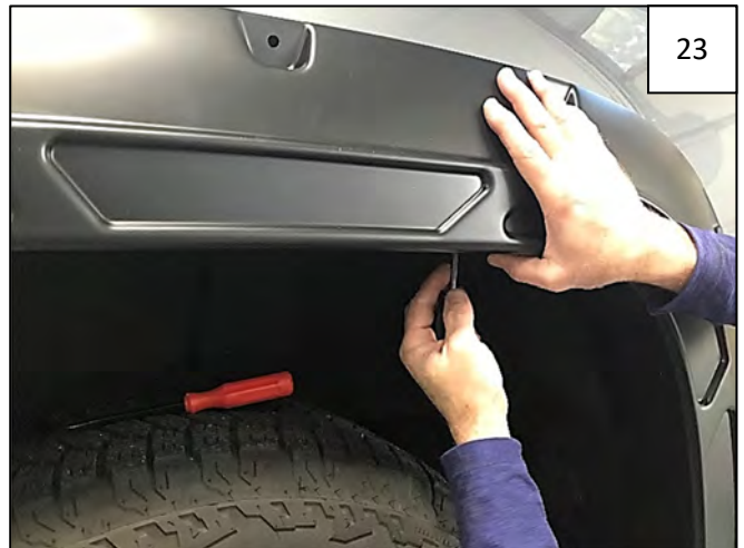
Apply pressure to flare towards vehicle body at each fastening point and tighten all screws.
