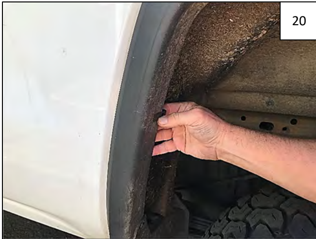
Remove fasteners installed in Step 17 and remove flare from fender. Slide a supplied Long "U" Clip over each mark made in Step 18.
