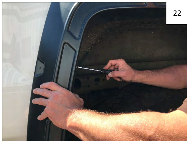
Install supplied #10 Truss Head Screws through holes in flare and into clips installed in Step 20.
