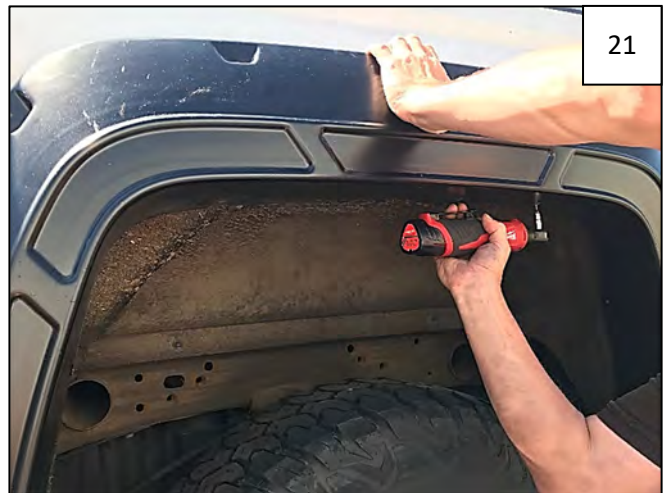
Hold flare on fender and reinstall T15 fasteners.
