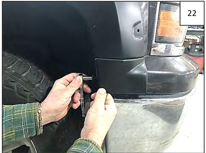
If your truck is a 2014-2015 1500, reinstall 7mm bolt removed in Step 12 through flare and into factory hole.
