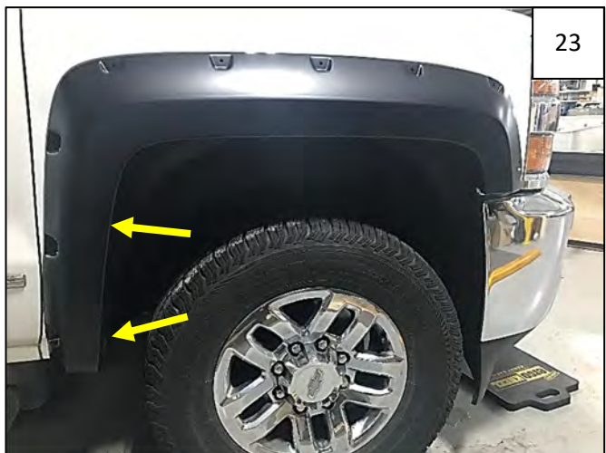
Reinstall 2 factory screws into holes at rear of flare, shown by arrows.
