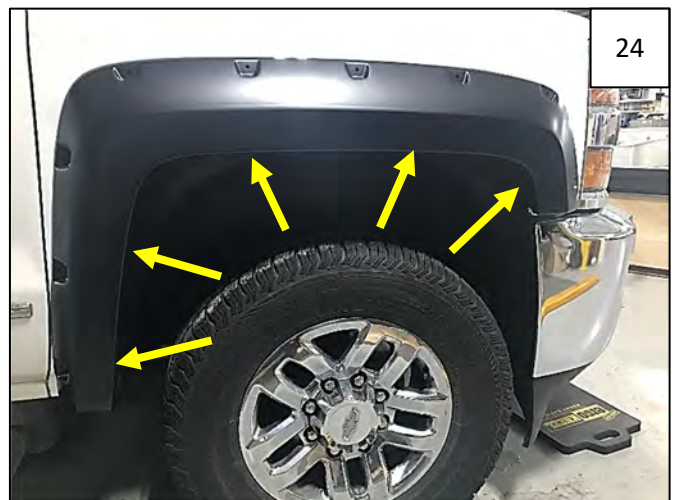
Apply pressure to flare towards vehicle and tighten all screws. Completed Front Flare Installation for 2015-2019 Chevy 2500, 3500.
