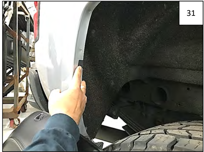
Remove flare from fender and peel liner from supplied Foam Tab. Center 5 foam tabs over marks made in Step 29, folding over wheel well lip.
