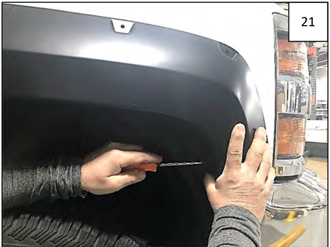
Install supplied Short Screw into "S" Clip installed in Step 19.
