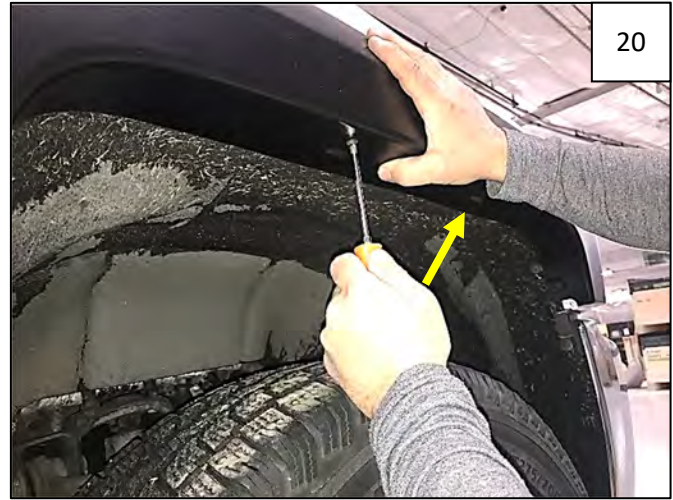
Holding flare firmly on fender, install 2 supplied #10 Truss Head Screws through topmost holes in flare and into Inner Bracket Clips. NOTE: Inner lip of flare should go over Inner Bracket installed in Steps 14-16. Do not tighten.
