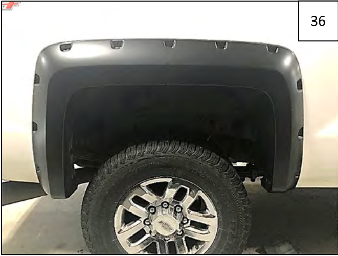
Completed Rear Flare installation.
