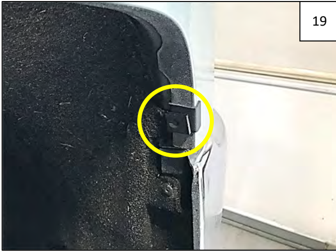
Install supplied "S" Clip over foam tab.
