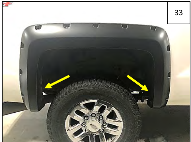
Hold flare on fender and install lowermost factory screws as shown by arrows to hold flare in place.
