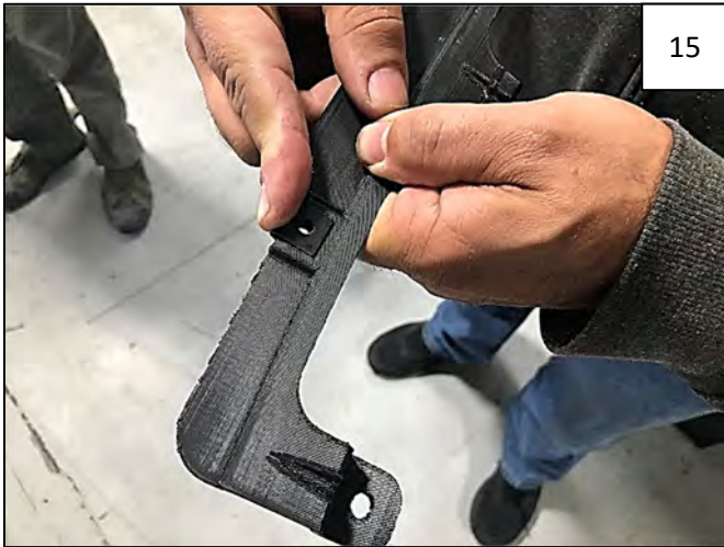
Attach 2 supplied Short "U" Clips to the supplied Front Inner Bracket as shown.
