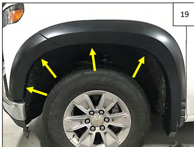
Align flare on vehicle and start 4 supplied Truss-Head Screws through holes in flare and into fender as shown.
