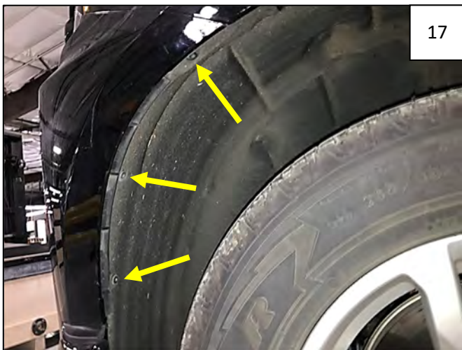
Remove 3 T15 Torx bolts from front bumper in locations shown by arrows – do NOT remove middle bolt. Retain bolts for use in Step 18.
