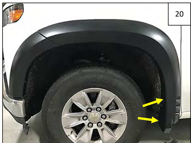
Start 2 factory T15 Torx screws at bottom rear of wheel well as shown. Apply pressure to outward face of the flare towards the center of the vehicle and tighten all screws.
