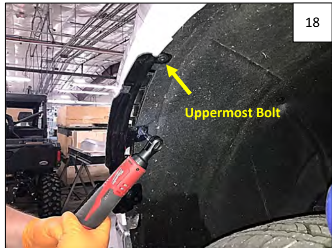
Install Front Inner Bracket on fender using 3 Torx bolts removed in Step 20, starting with uppermost bolt.
