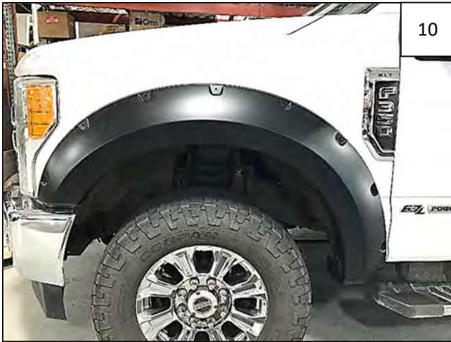
Completed Front Flare Installation.
