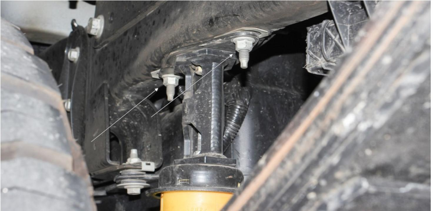
2. With the bump stop bracket removed, remove the factory studs/clips from the frame. Use screwdriver to disengage the clip and slide them downward and inward to remove.
