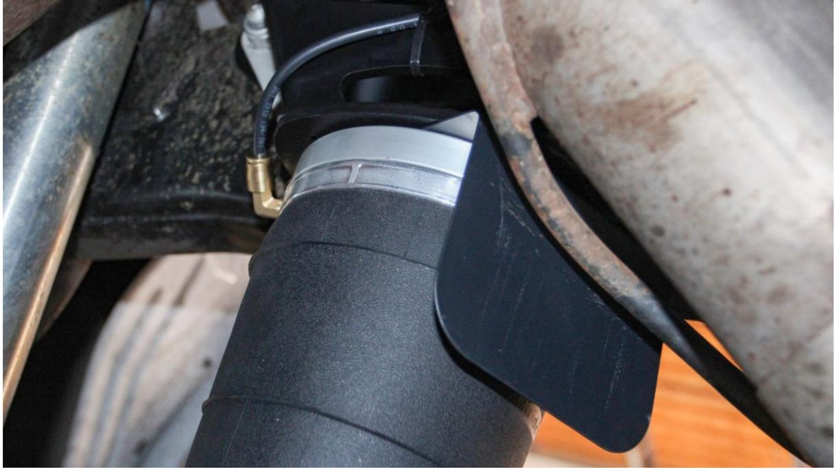
17. Remove the axle breather and use it to install the supplied Carli lower brake line axle bracket. Use the provided clips to secure the Carli Stainless brake lines to the Carli Bracket. If not running Carli rear lines, use the factory clips to secure the brake lines to the bracket.
