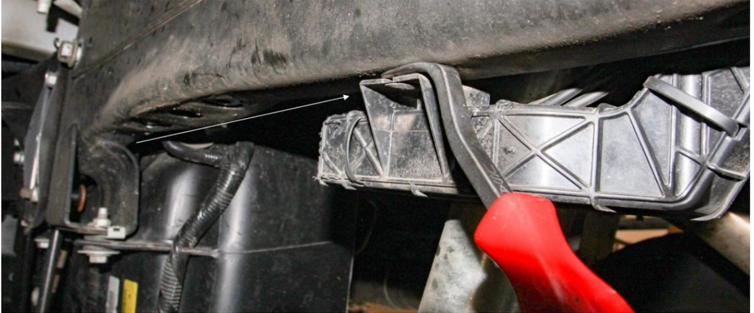
6. Slide the provided captured-nut bracket into the frame in place of the studs that were removed (that retained the factory rear bump stops).
