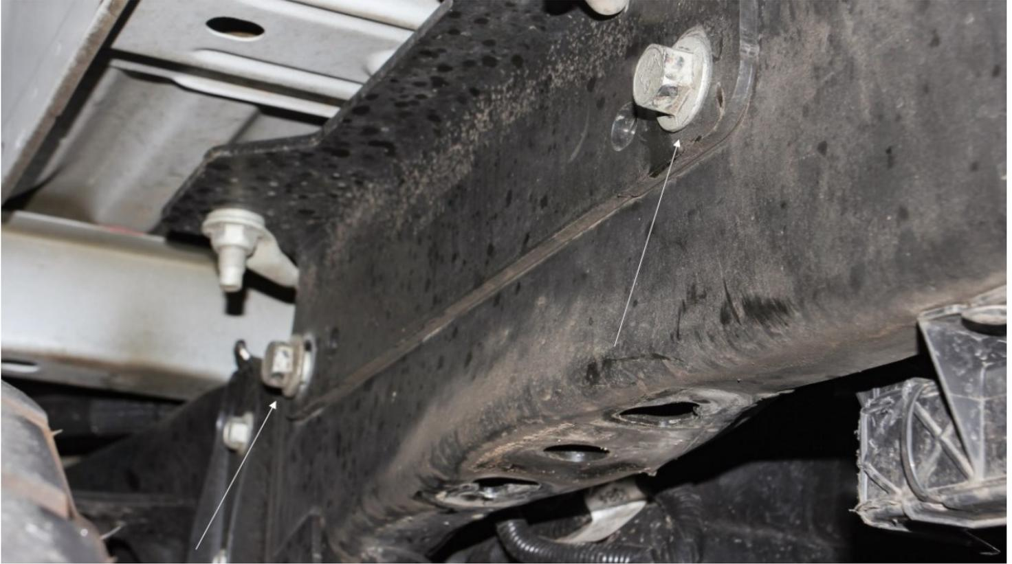
4. Using a 13mm socket, remove the 2 bolts securing the upper brake line bracket to the inside of the frame rail.
