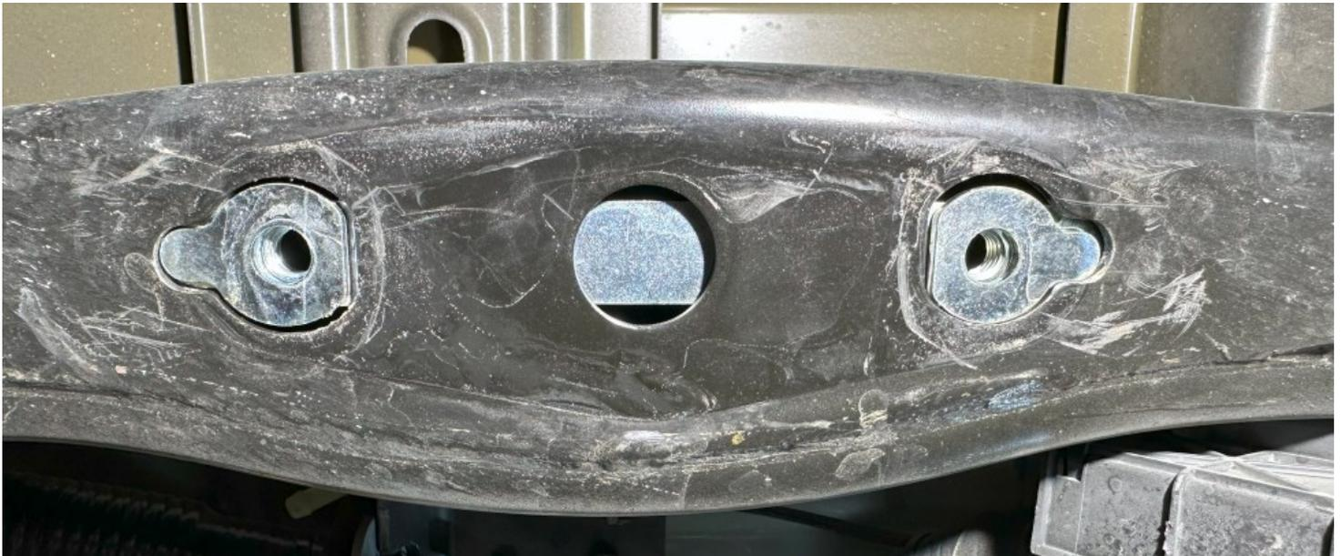
7. Slide the DRIVER Upper bracket (5 holes) into place on the INSIDE of the frame rail between the brake line bracket and the frame. Use the provided (qty. 2) 3/8"-16 x 1.25" bolts, split lock washers and flat washers to loosely secure the upper bracket, vertically, to the capture nut bracket inserted into the frame in the factory bump-stop location.
