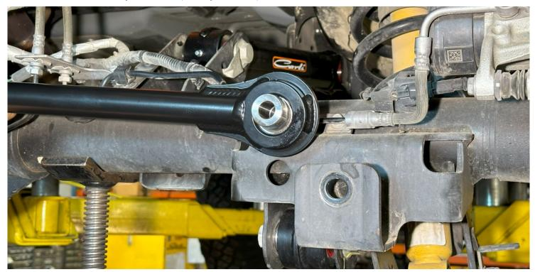
11. Install the adjustable end into the frame bracket and secure with the factory hardware. *You may need an assistant to push on the axle to line up this bolt hole.*
