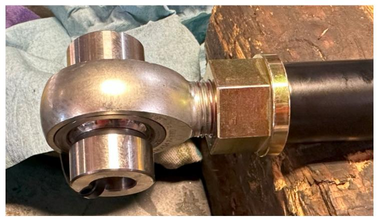
9. With everything torqued, remove the bar from the vice and CONFIRM the ends remained parallel. Any adjustments can be made by putting the fixed end back in the vice and clocking the adjustable end with a large adjustable wrench even with the jammit-nut tight (before the Loctite sets). Just be sure the jammit-nut doesn't loosen during the re-clocking, if necessary.
