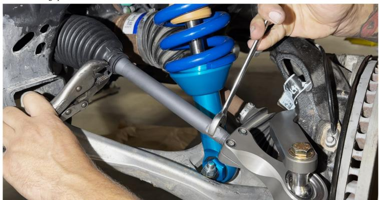
6. 1/4" 12-Pt Socket — EVENLY tighten the bolts securing the tie-rod end to the tie-rod. Torque to 14lb/ft.
