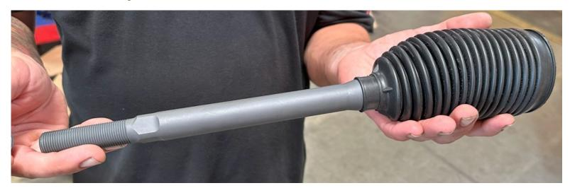
11. Thread the outer tie rod end onto the tie-rod. No anti-seize or Loctite is needed here as the graphite coating on the tie-rod is a dry-lube.
