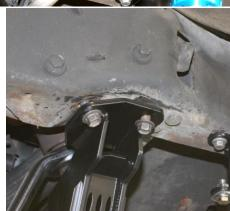
4. Once a few threads are engaged into the frame capture nuts, insert the captured bolt from the back side of the motor crossmember, through the track bar bracket and secure with the factory nut in the recess of the bracket.
