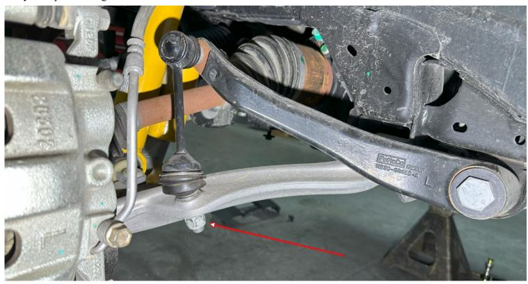
4. **6mm Hex Driver & 21mm Wrench** — Loosen the nut on the tie-rod end so it's only engaged a few threads. Use a tie-rod separator to unseat the taper, then remove the nut and disconnect the Tie-Rod from the Steering Knuckle.
