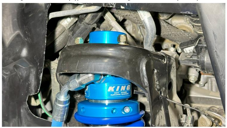
16. Index the lower T-Bar of the coilover to the angle of the lower arm and secure with the provided hardware. The 14mm/12mm Reducer Sleeves will go into the arm first, then, from the bottom, insert the M12-1.75 x 80mm Bolts with a washer on the head through the arm/reducer sleeve, and t-bar and secure with a washer and nut.
