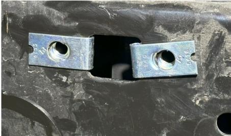
3. Use the provided 5/16" bolts and washers to secure the mounts to the Driver and Passenger side, respectively.
