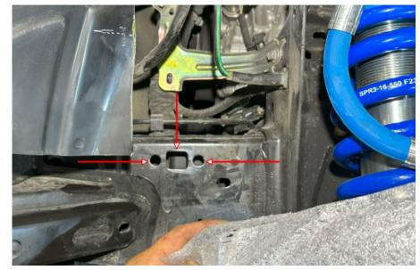
2. Through the center hole, slide the captured U-Nuts into position so the threads are centered to the outer 2 holes.
