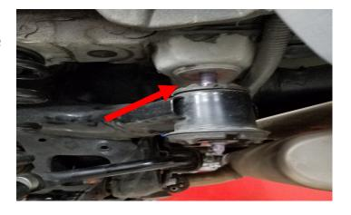
Add the ReadyLift 1" aluminum spacers to the front cradle mounting locations, use the provided hardware M16 bolts, washers, laser cut 2" washer, and the OEM dust shield. Snug these bolts but do not tighten.
