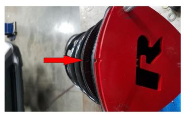
Install the completed strut assemblies into the strut tower using the factory hardware. When installed the R logo so that it is legible from the wheel. Do not tighten at this time.
