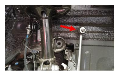
Support the lower control arm with a suitable jack. Remove the two strut to knuck-le bolts.
