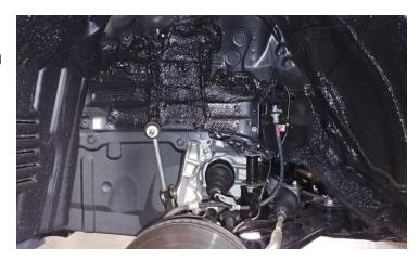
Add the ReadyLift strut spacer to the OEM strut, there is a dot on the OEM strut assembly align the notches on the spacer with this dot. Use the provided hardware M10 flange nuts to secure the spacer to the strut. Torque to 30 ft-lbs. This Alignment is very important for camber correction.
