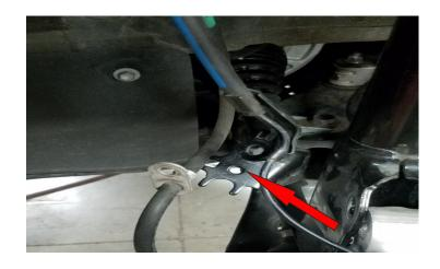
Unclip the ABS plastic bracket from the lower strut assembly. Remove the fastener that holds the ABS sensor to the steering knuckle. Remove the ABS sensor from the steering knuckle, and move the wire assembly to a position where it will not be pulled on when the strut is removed.
