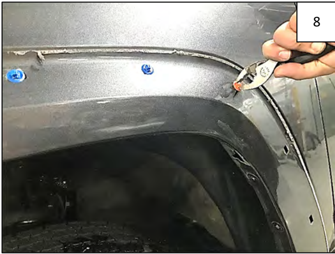
Use a vise grip or pliers to remove 1 factory clip as indicated by circle in Step 7, pulling with a rocking motion.
