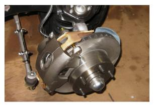
27. Temporarily mount the front wheels to observe for severe "toe-out" in the wheel positioning. If needed, loosen the two nuts on the tie rod adjusting sleeves and turn them approximately 2 to 2.5 turns or until wheels appear straight. This will temporarily adjust the toe in of the vehicle to enable you to drive the vehicle to an alignment shop. Tighten the tie rod clamp bolts.
