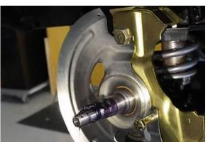
21. Install the tie rod end into the steering arm on the new spindle, tighten and torque the nut to 35 ft lbs. Install a new cotter pin.
