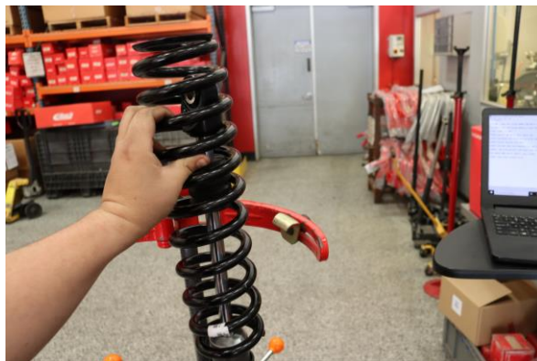
Step 13. Remove OE main spring.
