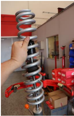
Step 20. Install Eibach main spring.
