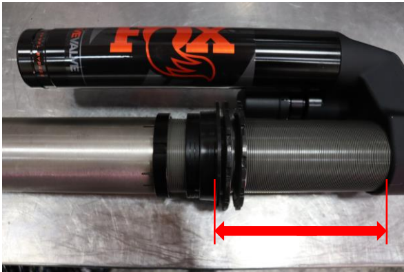
Step 15. Set pre-load to 190mm (7 1/2in.) from bottom of spring seat to bottom of furthest point on reservoir bridge. (Reservoir bridge is not flat relative to spring seat. Be sure to measure from the side opposite the reservoir).
