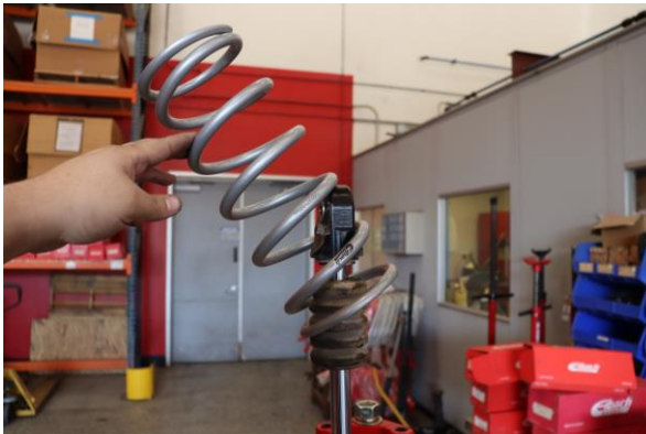
Step 17. Install Eibach secondary spring.
