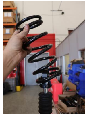
Step 14. Remove tender spring.
