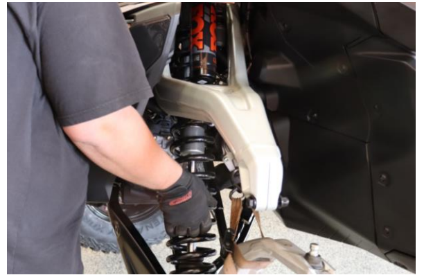
Step 10. Remove shock assembly from vehicle between upper and lower control arms.
