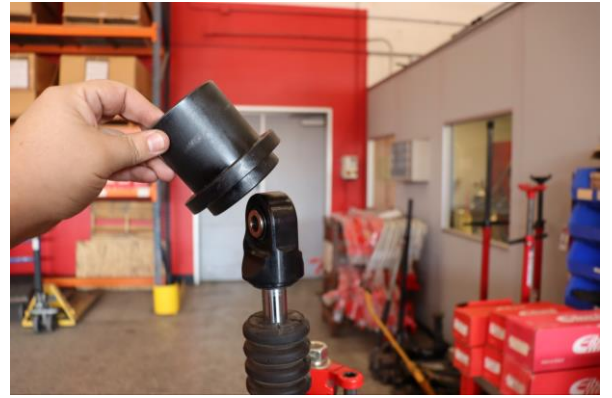
Step 19. Install OE spring slider with larger face pointed away from secondary spring.
