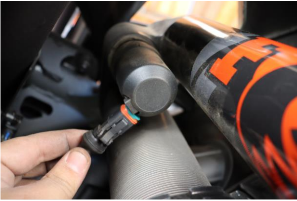
Step 25. Connect the upper shock wire harness at the shock assembly.
