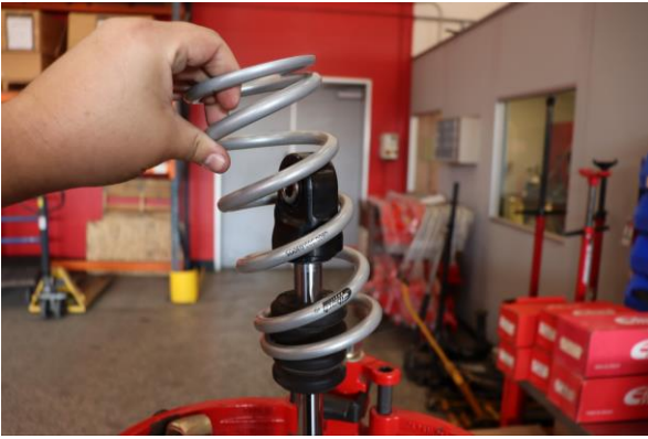
Step 18. Install Eibach secondary spring.
