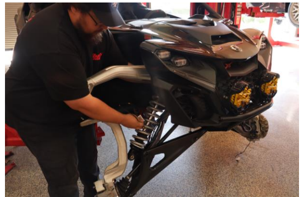
Step 23. Install shock in vehicle using upper mount bolt to hold assembly in place.
