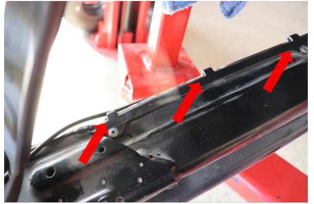
Step 26. Connect the lower shock wire harness and route through clips along lower trailing arm.
