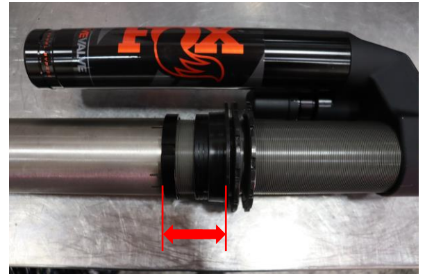
Step 16. Set crossover ring to 110mm (4 11/32in.) from bottom of spring seat to bottom of crossover ring.
