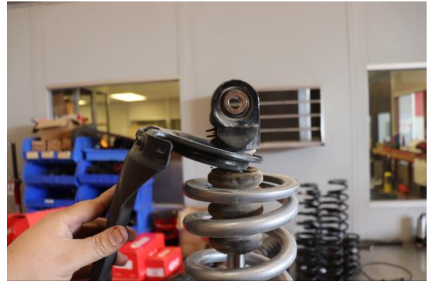
Step 20. Install lower spring retainer. Decompress spring assembly making sure that lower spring retainer and main spring sit flush with lower shock mount.
