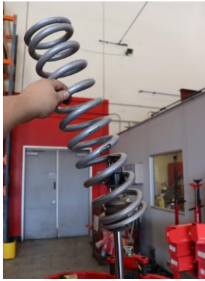
Step 19. Install Eibach main spring.
