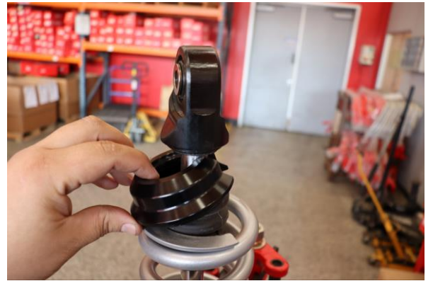
Step 21. Compress shock assembly enough to install lower spring retainer. Decompress shock and ensure spring and retainer sit flush on lower mount.
