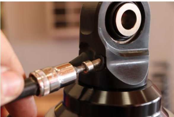
Step 11. Remove both 4mm allen head screws securing wire harness to lower shock mount. Remove wire harness from mount.
