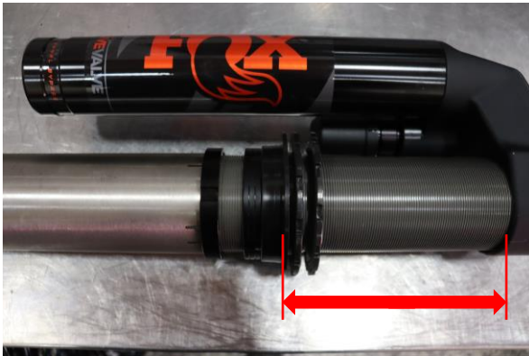
Step 15. Set pre-load to 215mm (8 15/32in.) from bottom of spring seat to bottom of furthest point on reservoir bridge. (Reservoir bridge is not flat relative to spring seat. Be sure to measure from the side opposite the reservoir).
