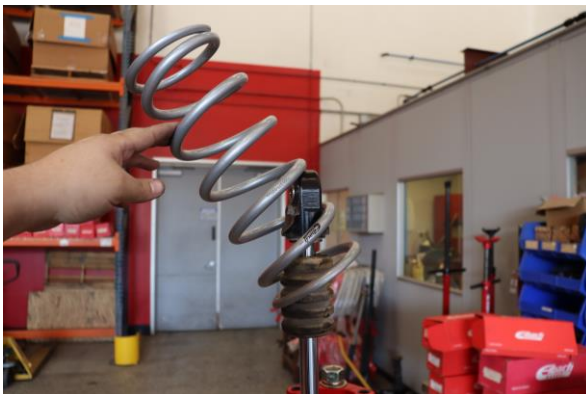
Step 17. Install Eibach secondary spring.
