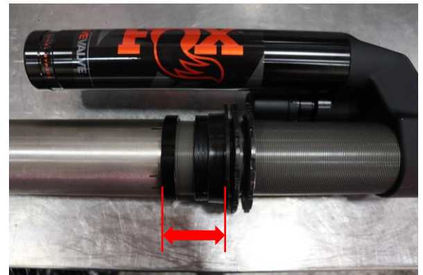
Step 16. Set crossover ring to 90mm (3 17/32in.) from bottom of spring seat to bottom of crossover ring.
