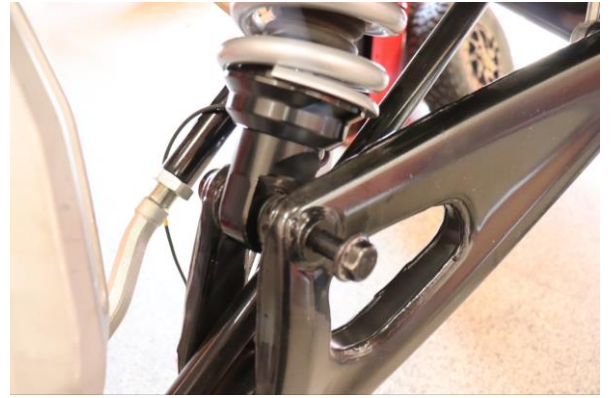
Step 8. Remove 21mm lower shock nut and bolt.
