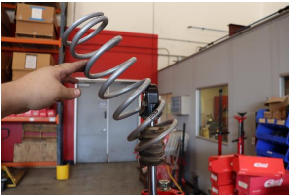
Step 17. Install Eibach secondary spring.
