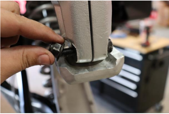
Step 7. Remove 15mm bolt and nut at upper control arm ball joint.
