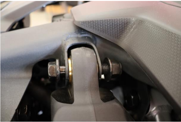
Step 9. Remove the 21mm nut and bolt from the upper shock mount. Move upper control arm up and carefully move spindle to the side.
