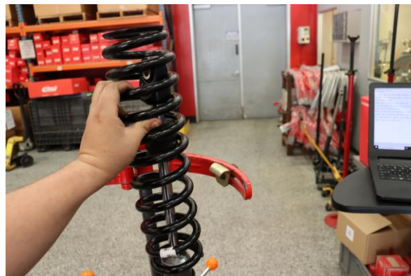
Step 13. Remove OE main spring.
