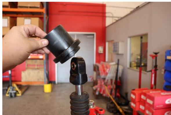
Step 19. Install OE spring slider with larger face pointed away from secondary spring.
