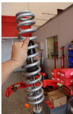
Step 20. Install Eibach main spring.
