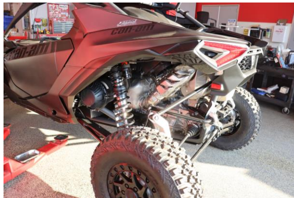
Step 29. Install wheels and tires with lug nuts snug, lower vehicle and torque lug nuts to manufacturer specification.
