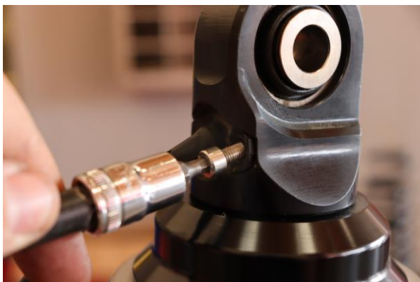
Step 22. Install lower shock wire harness in lower shock mount using both 4mm allen head screws. Tighten to manufacturer specification.
