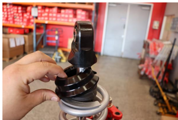
Step 21. Compress shock assembly enough to install lower spring retainer. Decompress shock and ensure spring and retainer sit flush on lower mount.
