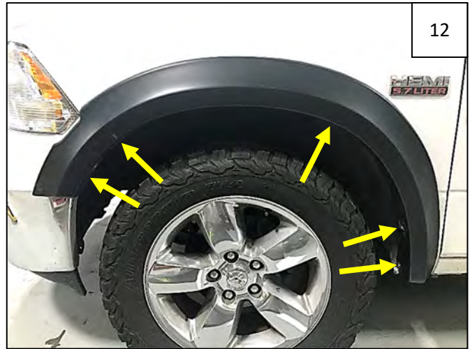
Hold flare on fender and start 5 factory fasteners at locations as shown.
