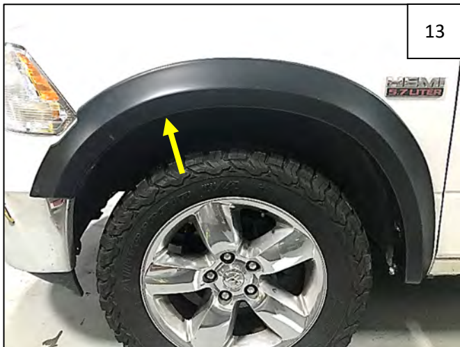
Install a supplied Truss Head Screw through fender flare and into clip installed in Step 10.
