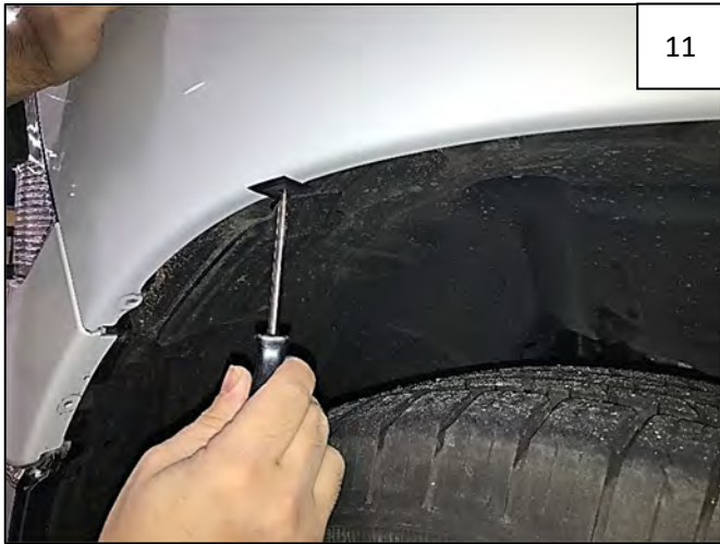
Use an awl to poke a hole in tab for ease of screw installation in Step 13.
