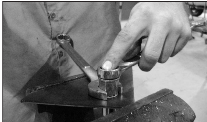
FIGURE 2 - 1/2" RIVET NUT SHOWN
