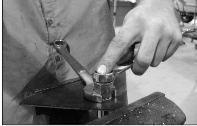
FIGURE 2 - 1/2" RIVET NUT SHOWN
