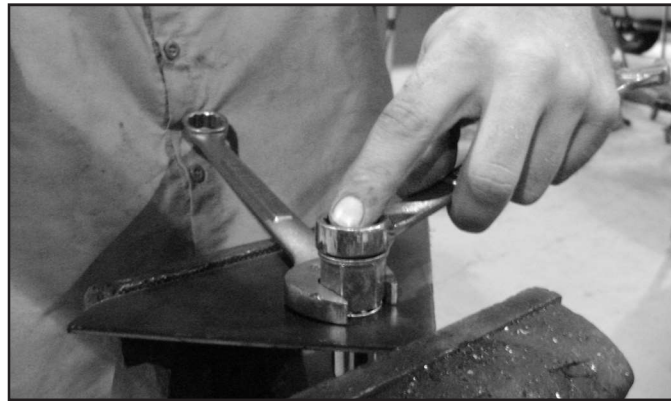
FIGURE 2 - 1/2" RIVET NUT SHOWN
