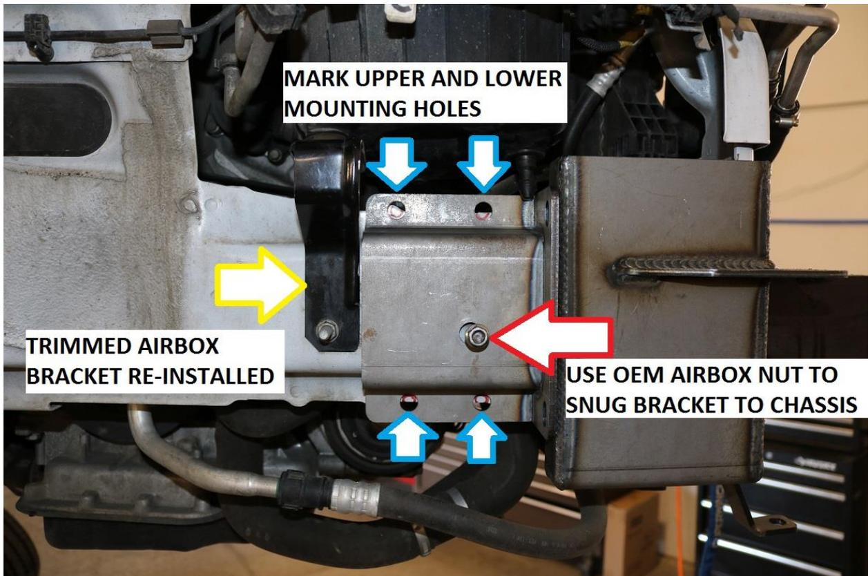
41) With the mounting holes marked, remove the bracket and use a dremel or die grinder with burr bit to notch out the hole mounting locations. See image below for reference of finished cuts.
