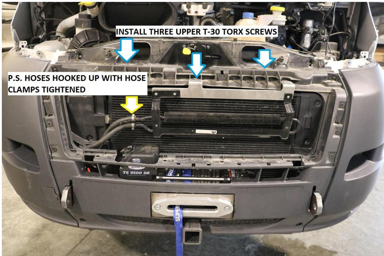
55) Perform any additional trimming of the grill to clear the winch and power steering cooler. Refer to the images below for reference on trimming around the Superwinch.
