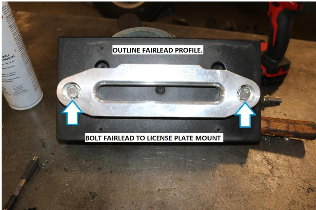
35) Test fit trimmed license plate mount by fully installing the fairlead onto the winch mount using the hardware provided with your winch. Ensure the bolts are installed from behind as there is very little room between the fairlead and the winch when installed.
