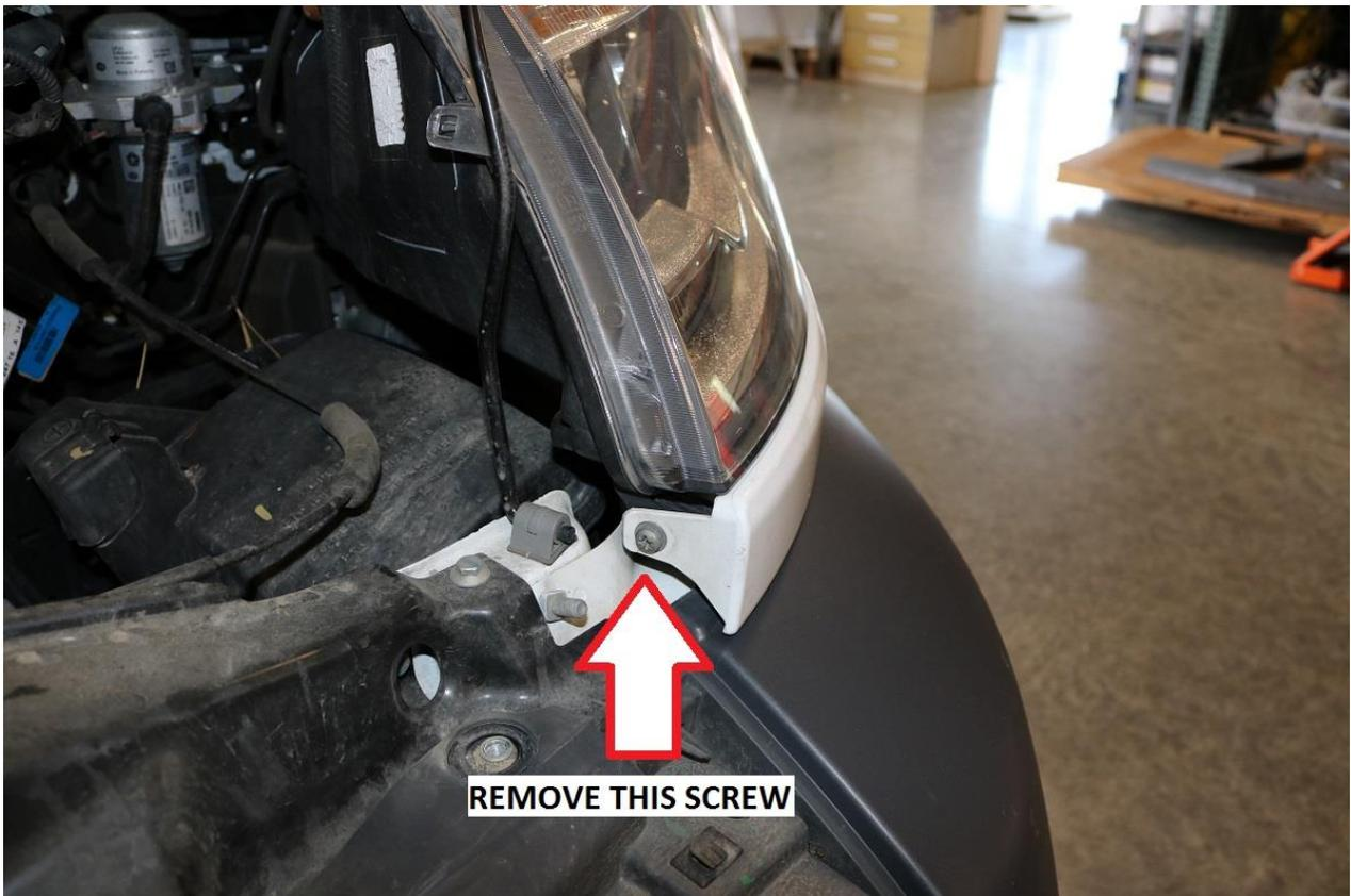
11) Pull the lower headlight trim away from the vehicle carefully. There are two trim clips towards the outer back edge of the head lamp. Try to support near this area as you pull away from the vehicle.
