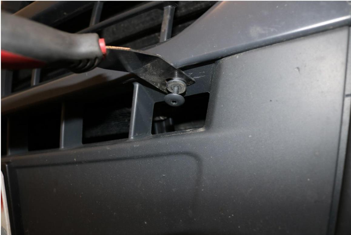
16) Remove the center grill by pulling it straight up and slightly outwards from the vehicle. There are two barb style plastic clips lightly holding it to the vehicle.
