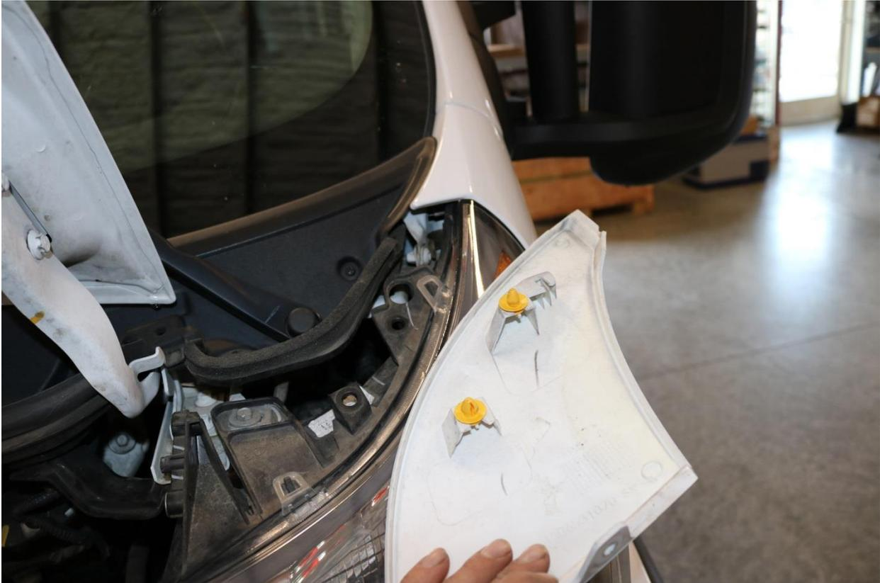
10) Remove the lower headlight trim panel by first locating the Phillips head screw along the inner edge of the headlight.
