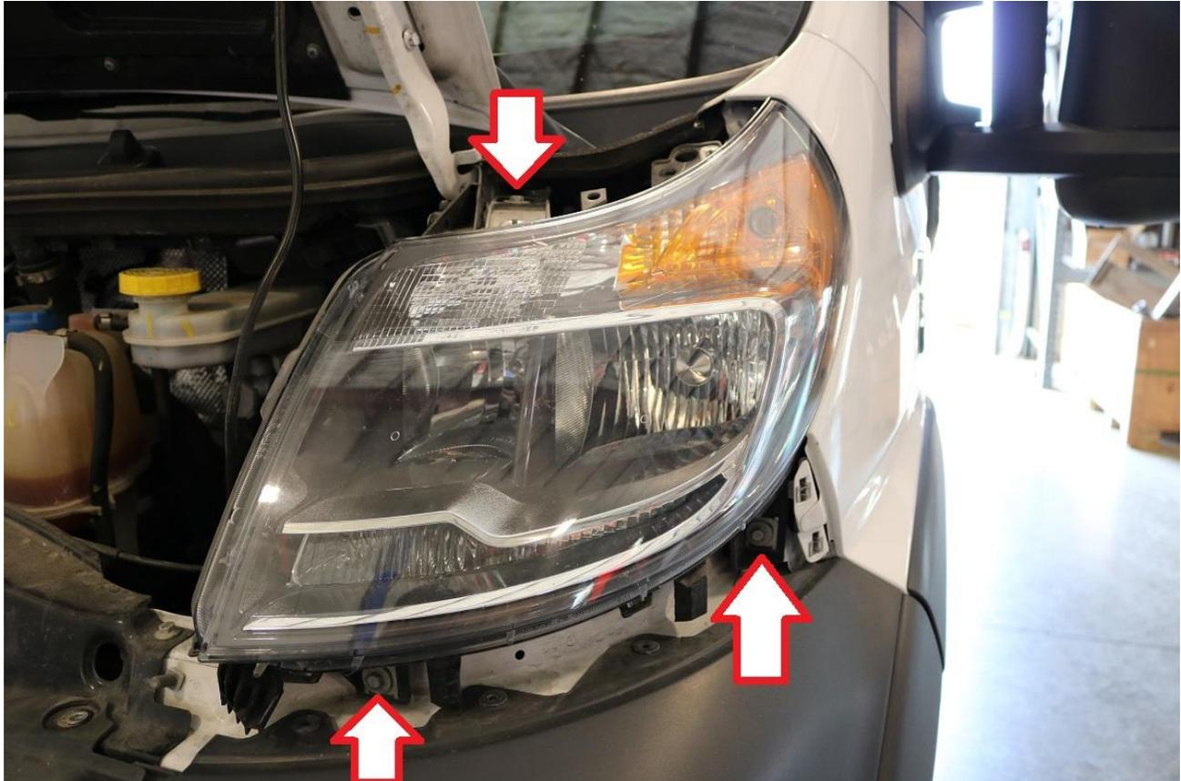
13) Once the three bolts are removed, pull the headlamp straight forward to unseat the push pin securing it to the vehicle.
