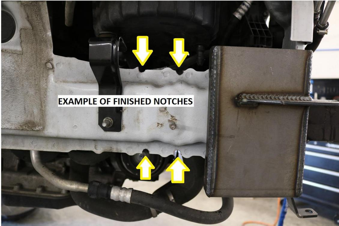
42) On the inside of the main chassis rail. Locate the threaded stud protruding towards the center of the vehicle. Use a small cut off wheel to cut this stud flush with the chassis. See image below for reference on stud location.
