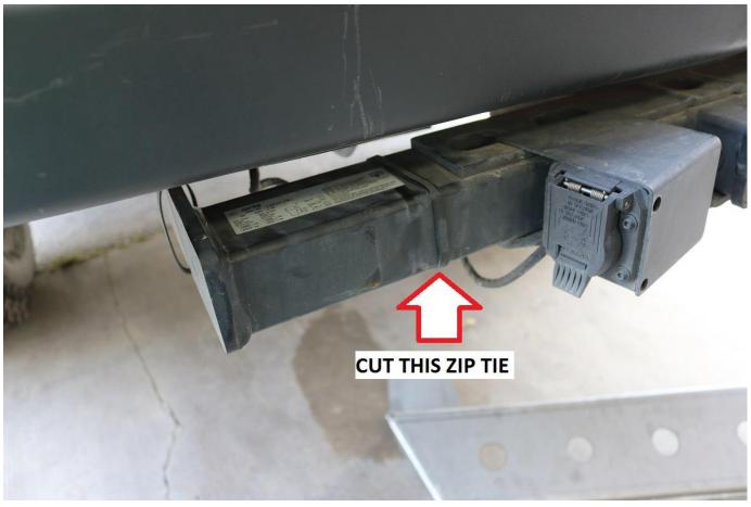
2) On the underside of the vehicle, locate where the wiring loops into the zip-tie on the side plate of the hitch. Pull this wiring out from the zip tie as shown below.
