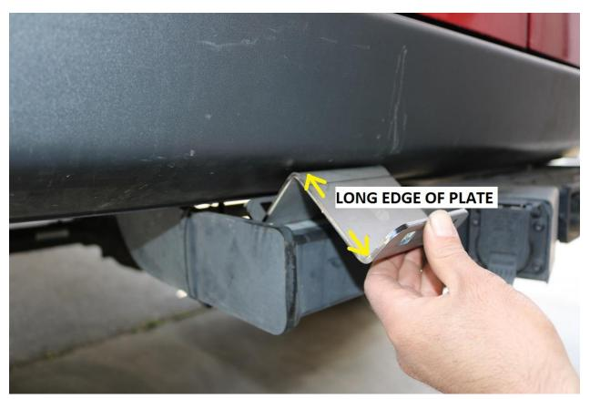
5) With the backing plates installed and slid as far over as it can be, insert the  $7/16-14 \times 1.0$ " long carriage bolts included in the kit from behind as shown. Just install the top bolts at this time.
