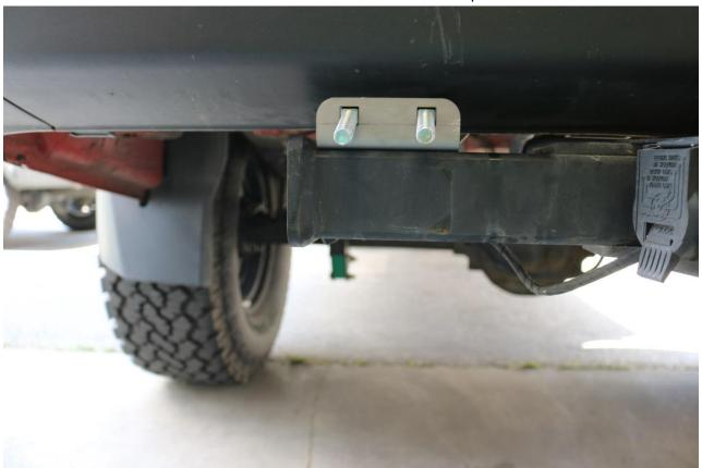
6) Position the rear hitch step in place as shown below. Install the bottom carriage bolts from below as shown so the bottom of the step has a smooth surface.
