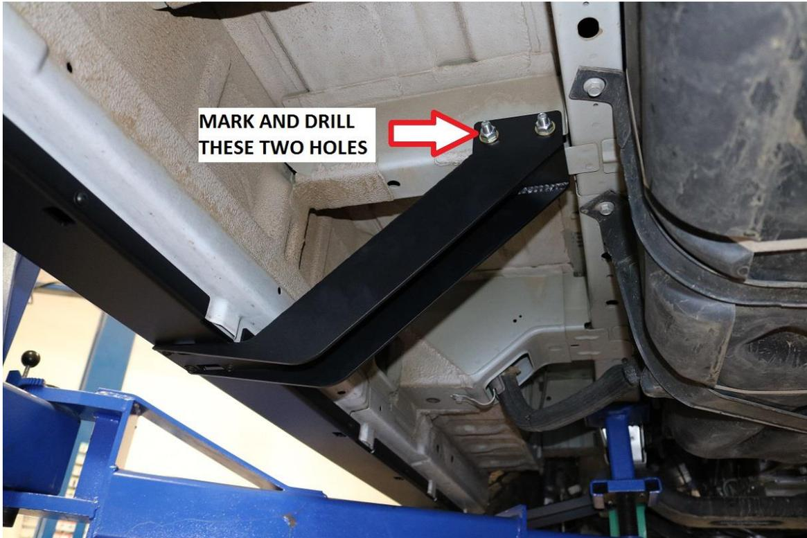
30) Torque the 7/16" x 4.0" bolts using a 5/8" socket / wrench to 30 ft-lbs (40 N.m)
