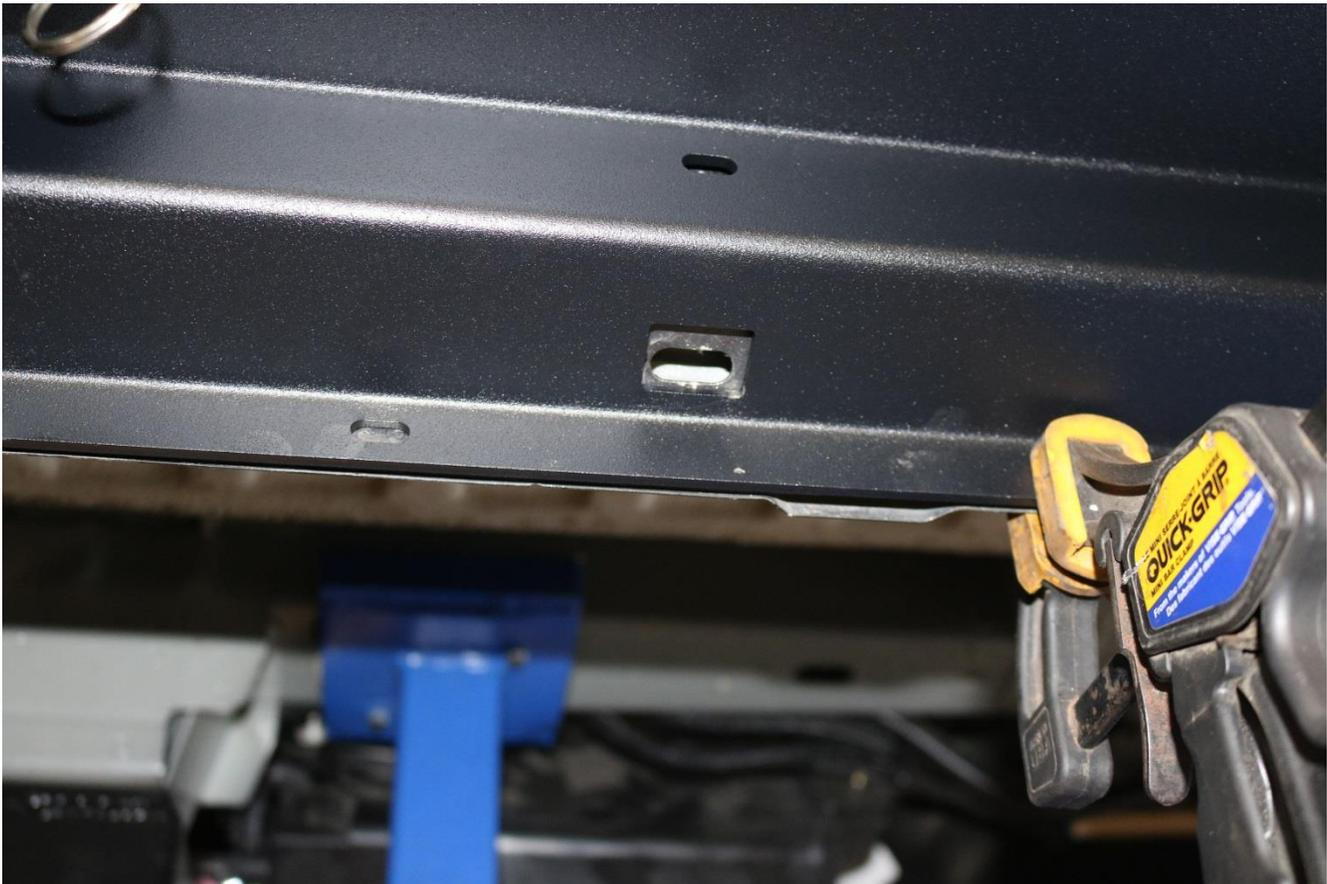
12) With the top plate in position, install the nut tabs as shown into the body. Use a ¼-20 button head with a flat washer under it to secure the nut tab to the chassis. Use a 5/32" allen wrench to snug the hardware. Do not fully tighten at this time.
