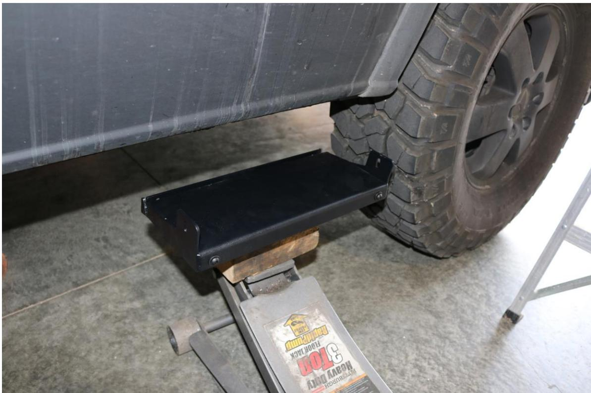
7) Install the inner bolts. Again be sure to use a washer under the head of the bolt.
