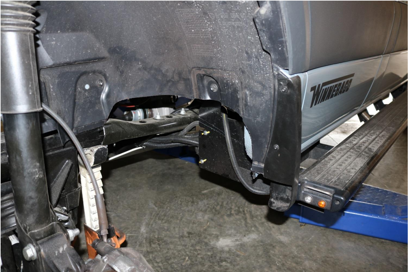
EXAMPLE OF COMPLETED CUT REAR HALF OF INNER FENDER LINER
