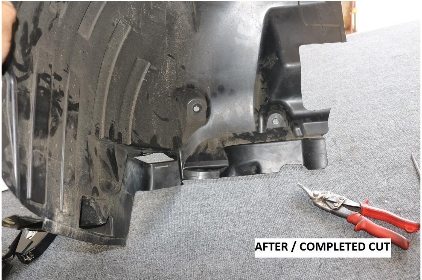
84) Trim the rear half of the fender liners as shown in the images shown below.
