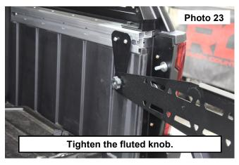
24. When closing the tailgate extension, place the fluted knobs back into the extension brackets.
