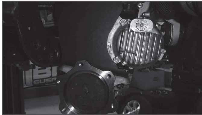
FIGURE 23 - SHOWN WITH DIFFERENTIAL ALREADY INSTALLED
