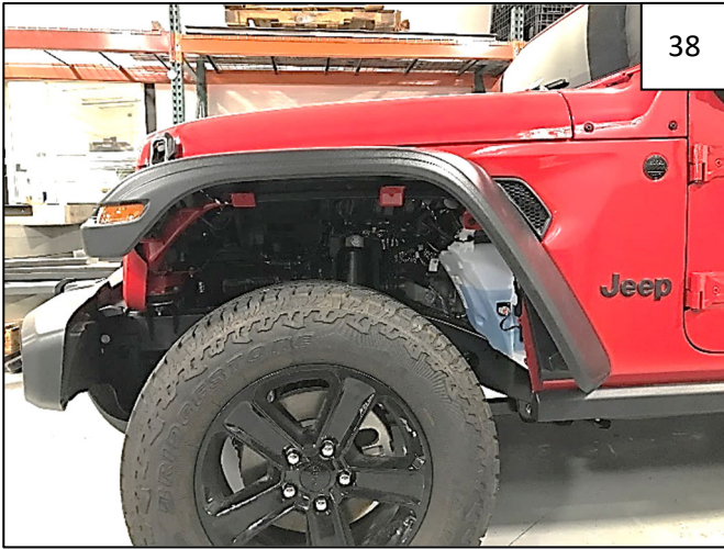
Complete Front Flare installation.
