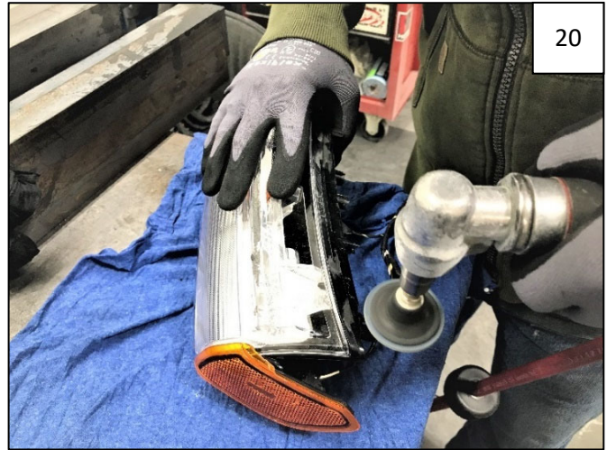
Using a sanding disc or sandpaper, sand down any remaining tab vestiges. Tab vestiges must be as flush as possible for proper installation.
