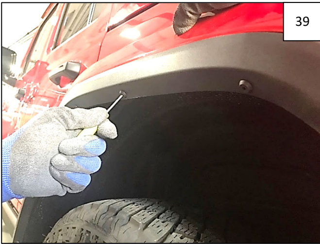
On rear factory flare, use an awl to pop 8 factory retainers in center of each retainer to disengage.
