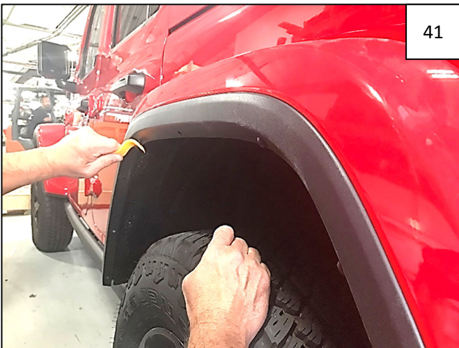
Using a plastic pry tool, pry each plastic retainer from vehicle and discard.
