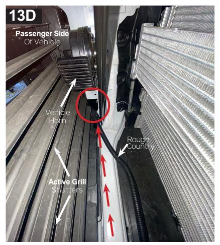
Route the ROUGH COUNTRY harness connector through the opening circled in red. You will pull the slack from the ROUGH COUNTRY harness from this area in the next step. Be careful NOT to interfere with the active grill shutters.
