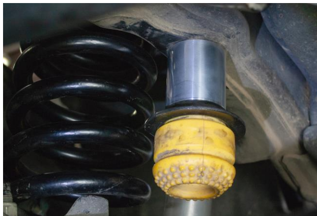
Figure 7: Assembled Bump Stop Installation
