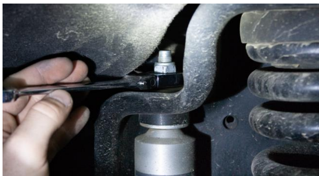
Figure 1: Front Shock Upper Nut Removal
