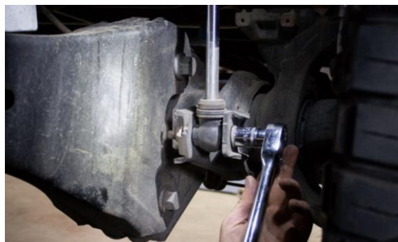
Figure 2: Front Shock Lower Bolt Removal
