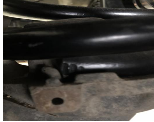
Figure 9: Bottom Spring Pigtail Installation
