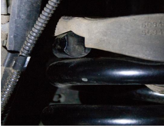
Figure 8: Top Spring Pigtail Installation
