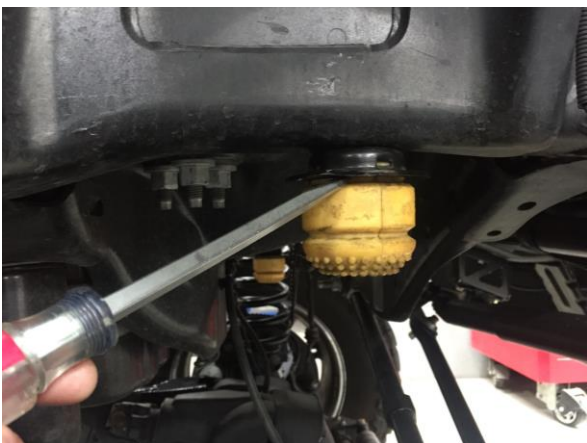
Figure 4: Bump Stop Spacer Removal
