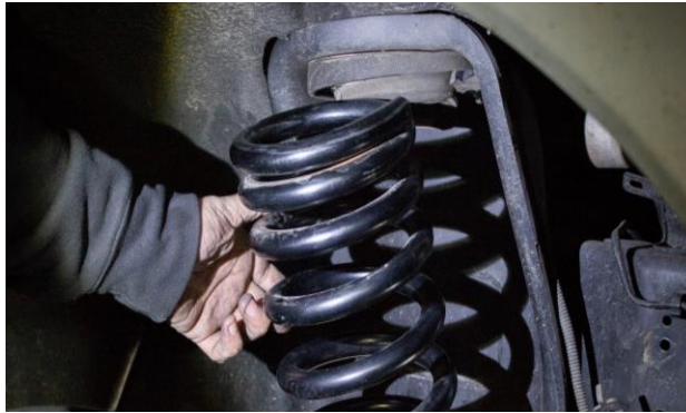
Figure 3: Front Spring Removal
