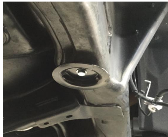
Figure 5: Bump Stop Mount Removal
