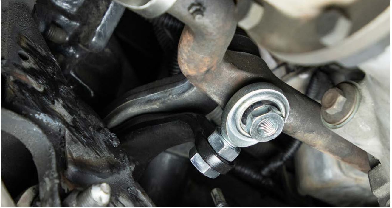
Figure 6: Pitman Arm Bracket Installed
