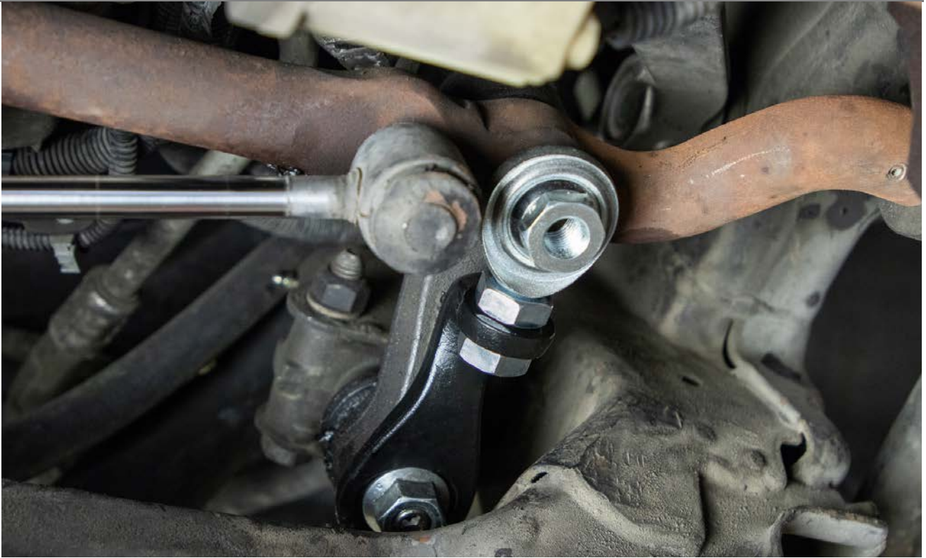
Figure 7: Idler Arm Bracket Installed
