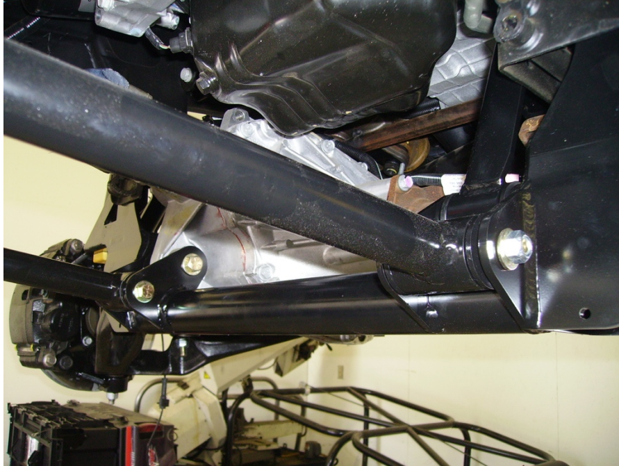
Figure 22: Attach 8033 compression strut tubes to 8071 crossmember
