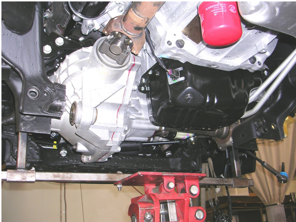
Figure 14: Factory crossmember and frame section removed.
