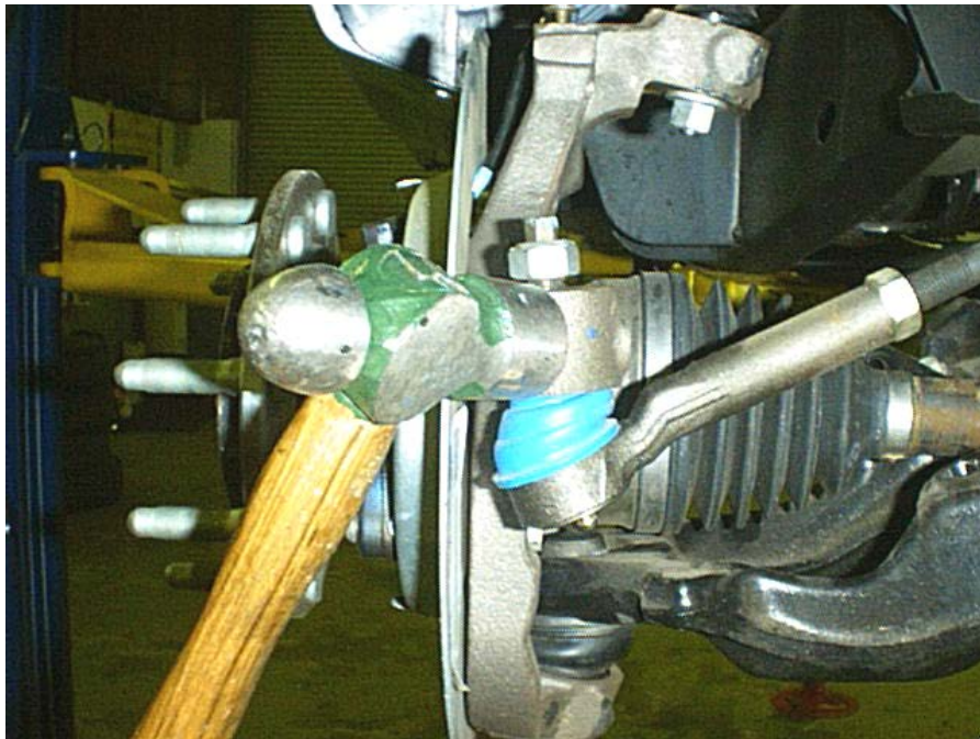
Figure 7. Remove tie rods from spindles.
