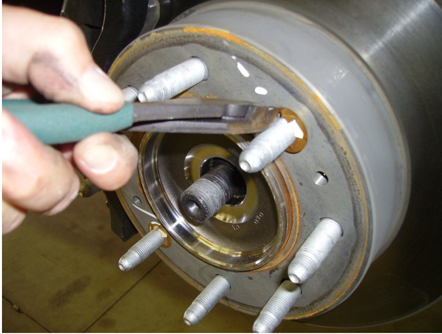
Figure 6: Remove clips from all 4 corners of vehicle. MUST DO for aftermarket wheels.
