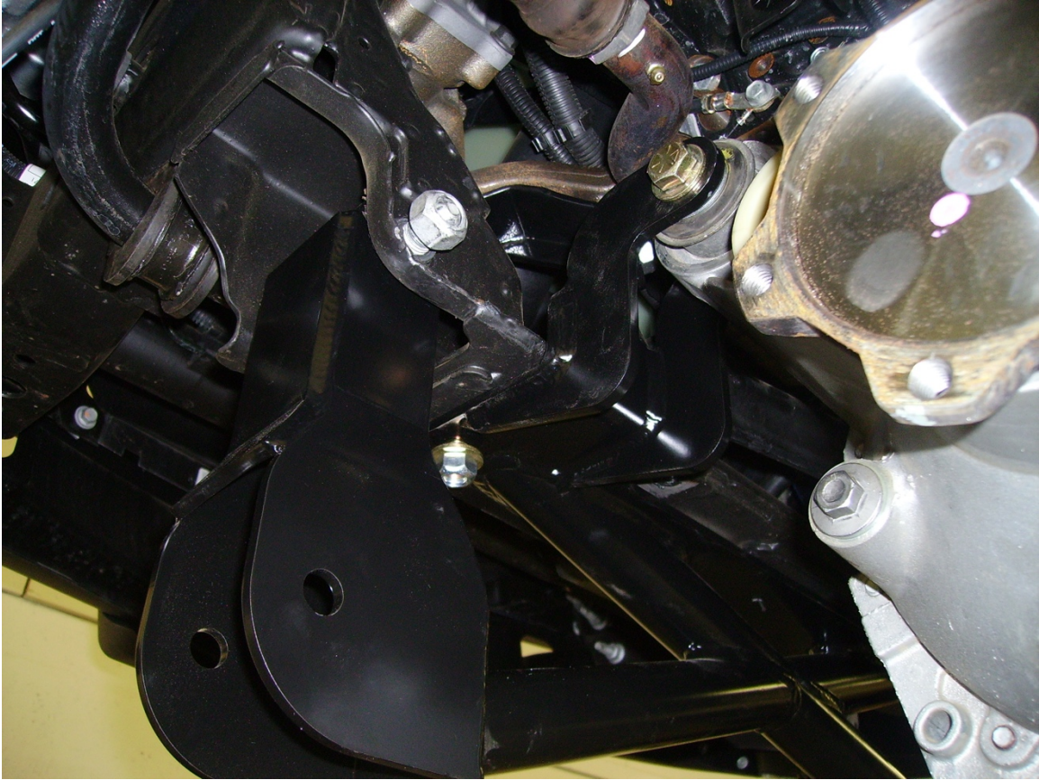
Figure 19: Front xmb and top mount on differential.
