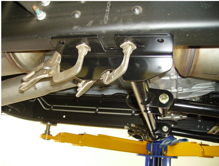
Figure 23: attach 8056 crossmember to 8053 compression strut tubes.
