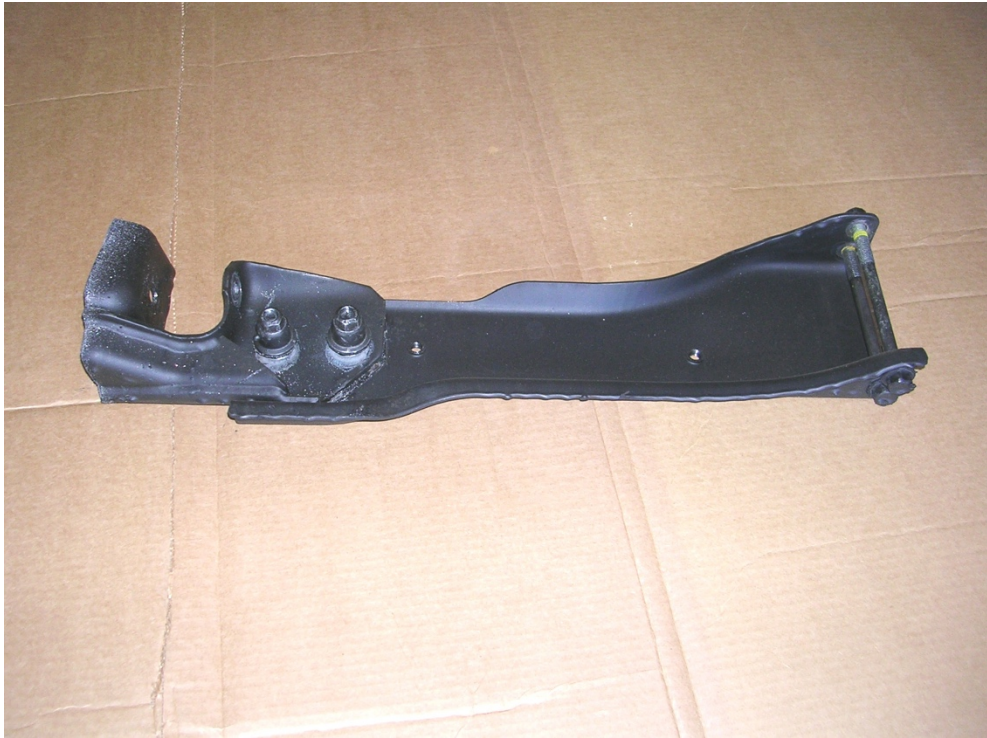
Figure 15: Factory crossmember and frame section removed.
