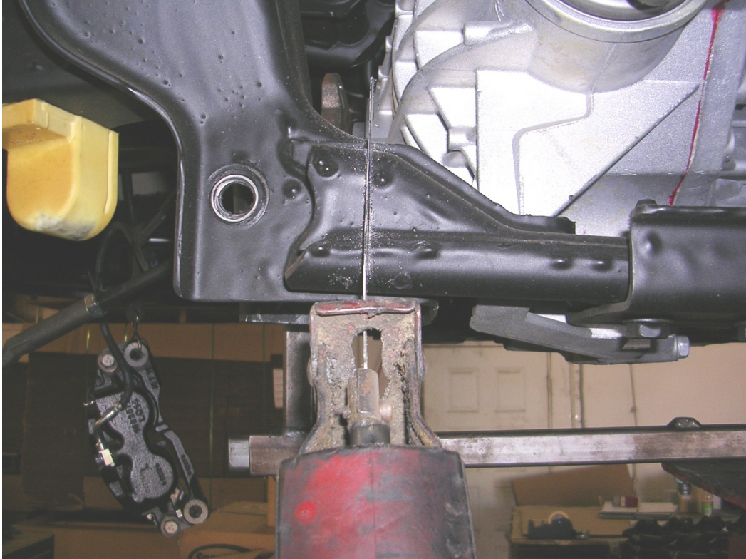
Figure 13: Cutting the frame pocket.
