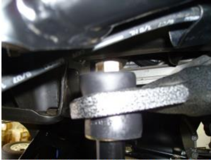
Figure 3: Bushings swell slightly when tightened properly. Don't over tighten.
