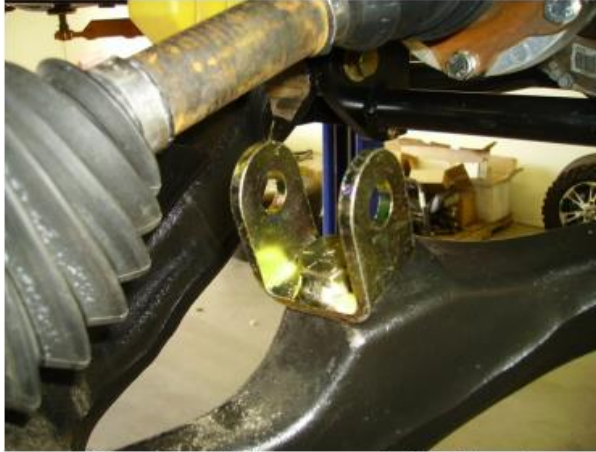
Figure 1: Clevis in lower a-arm, don't tighten yet.
