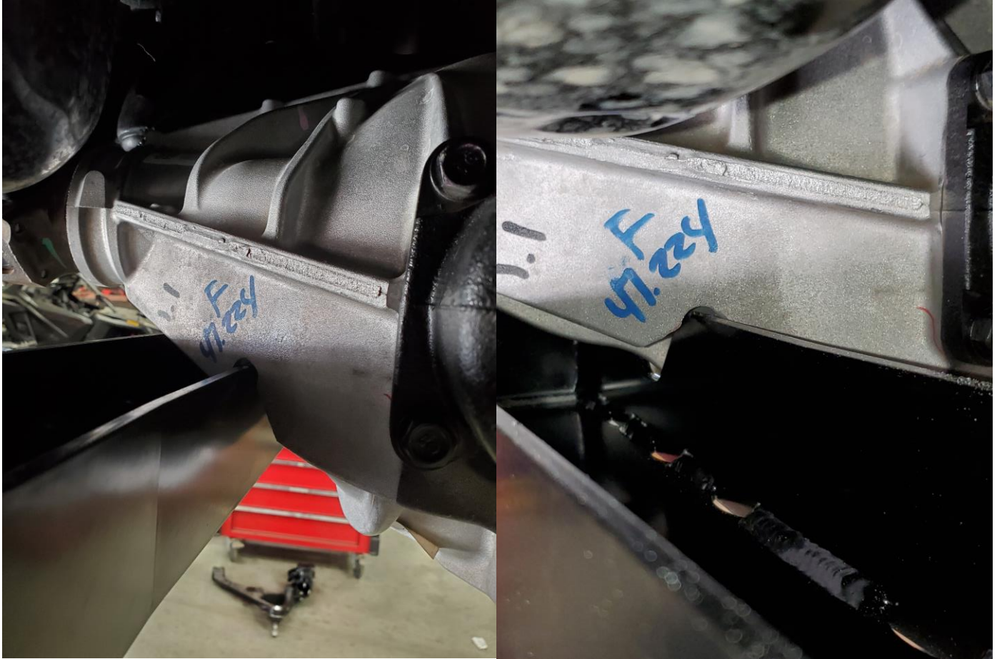
Figure 44: Clearance of rear crossmember.
