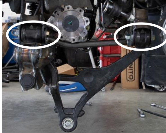
Figure 76: Lower Control Arm Bolts that do NOT get torqued at this step
