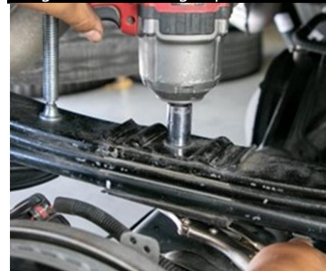
Figure 1: Removing Tapered Shim.
