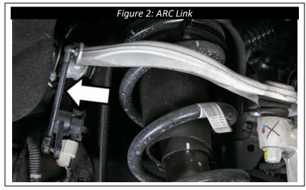
**4.** Support the lower control arms with a floor jack or stand. Prior to removing the upper control arms (UCAs), remove either sway bar end link to allow the lower control arms to cycle independently. Remove the strut to allow access to the upper arm pivot bolts.
