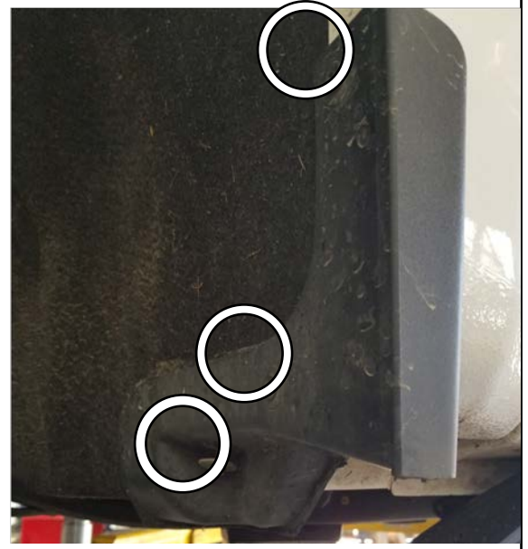
Figure 11: Plastic Mud Flap Trimmed and Reinstalled Chevy
