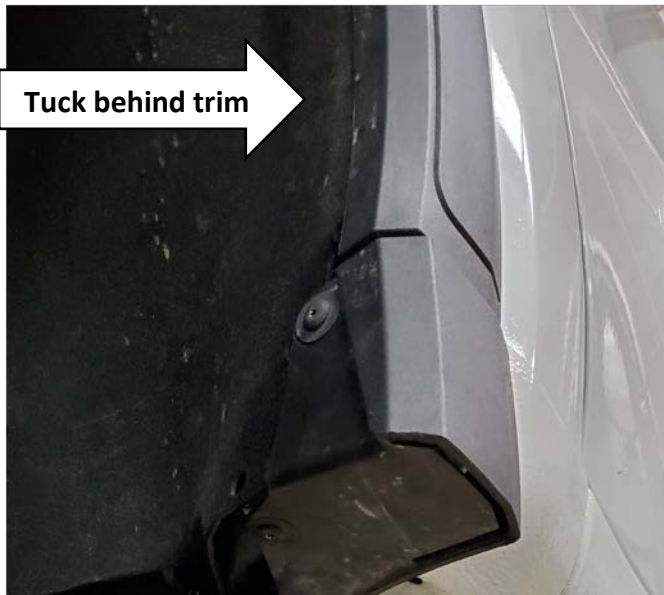
Figure 10: Plastic Mud Flap Trimmed and Reinstalled GMC
