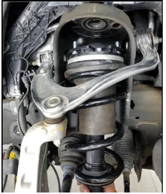
Figure 15: Install Strut Assembly into Vehicle
